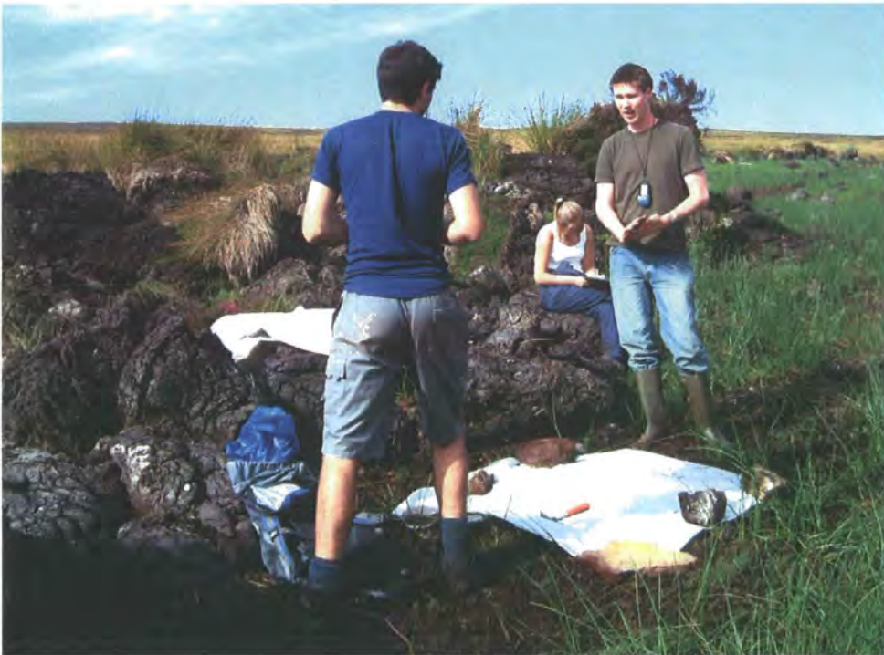
Figure 2.18 Setting a white plastic panel on a GCP and recording the location on a draft map
