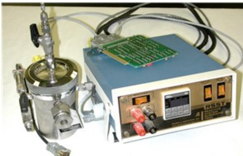
**Figure 3** Reactive System Screening Tool, with computer interface
