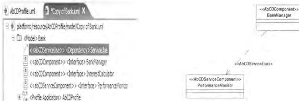
Figure 50 Dependency between BankManager and Performance monitor components using AbCDServiceUse stereotype
