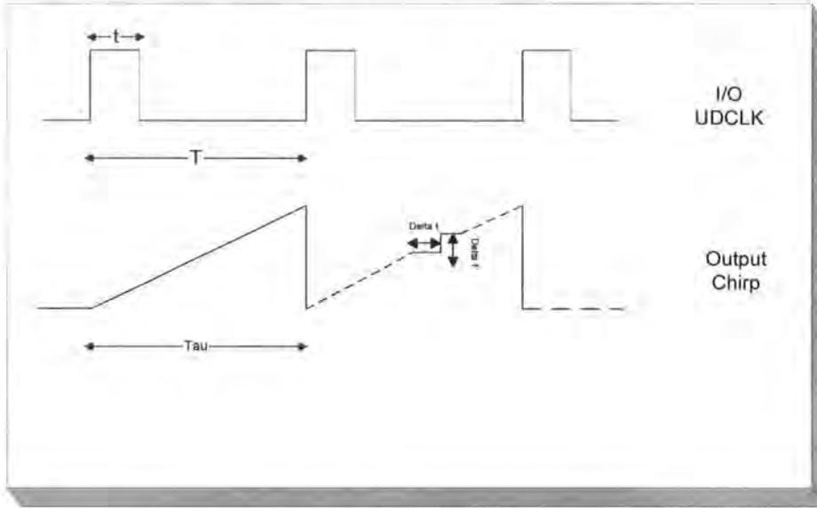
Figure 4.7: Relationship of I/OUCLK and Output Chirp
