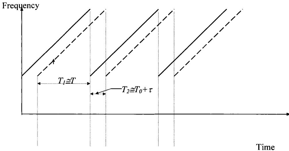
———— Transmitted chirp      - - - - - Received chirp
