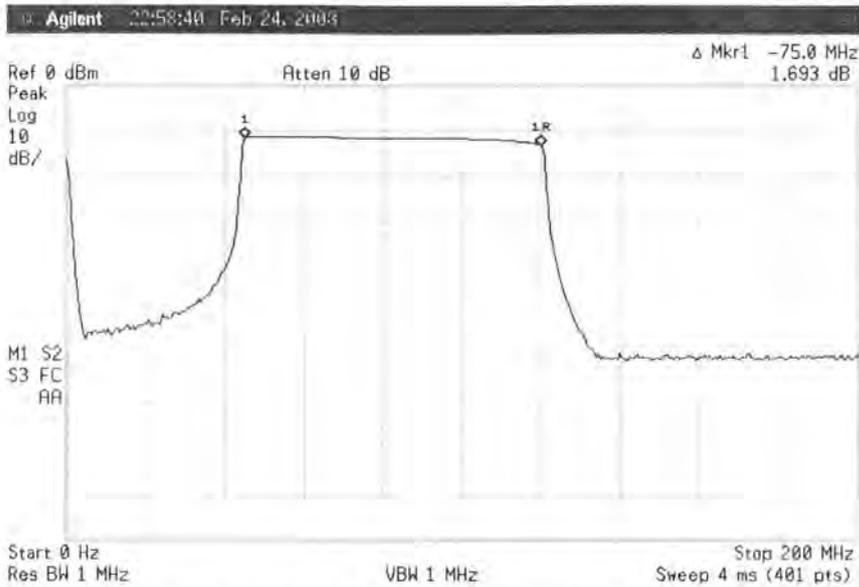
**Figure 4.9 AD9854 Output – 45/120 MHz**
