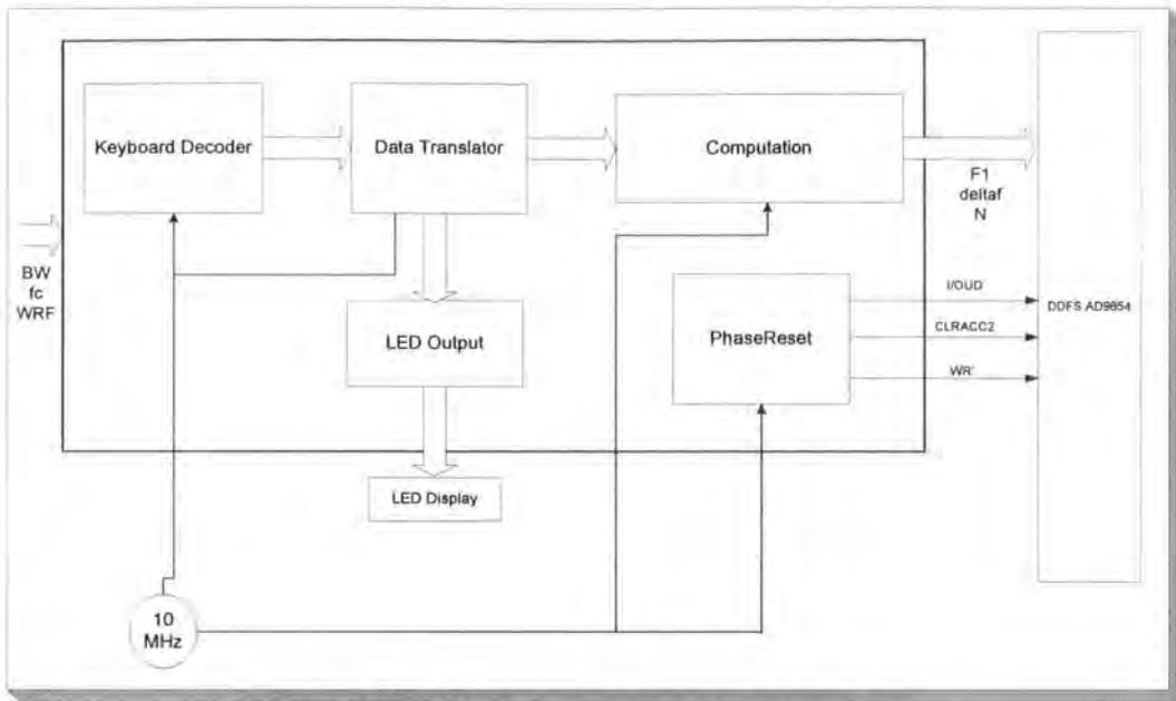
Figure 4.13 Modular Representation of Gate Array Design
