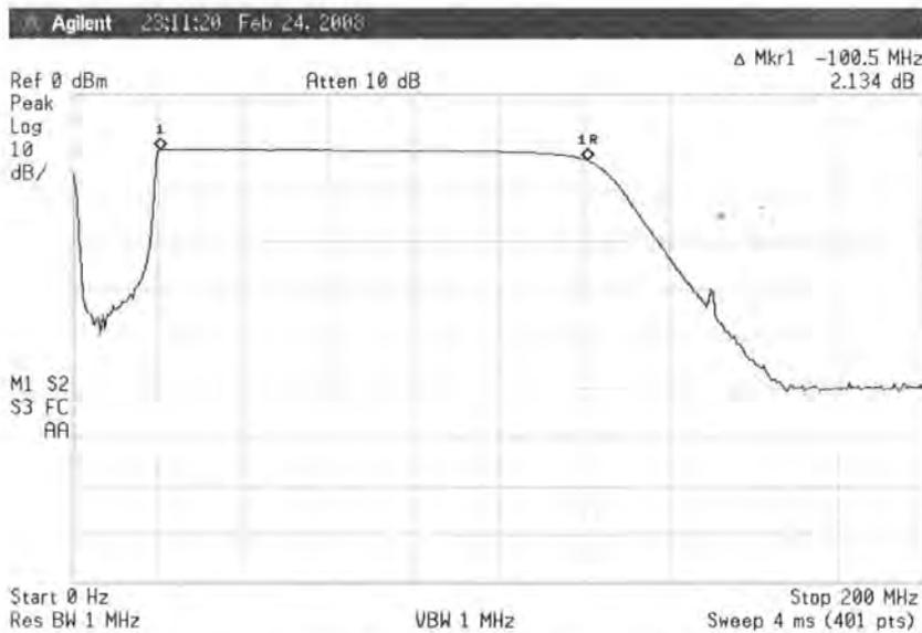
Figure 4.8 AD9854 Output – Wide Bandwidth (100 MHz)
