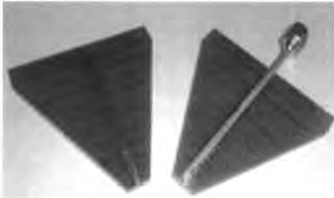
Figure 4.3: Log-Periodic Antennas (900-2600 MHz) [4]
