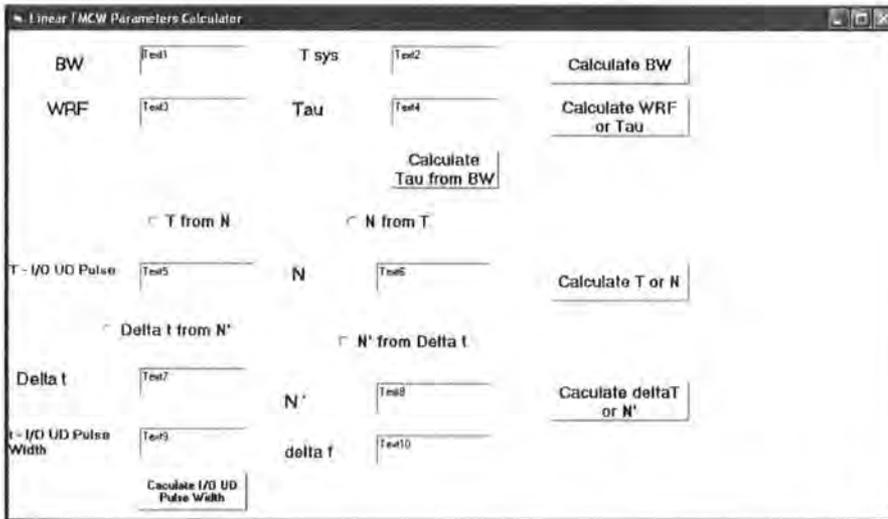
Figure 4.6: User Interface of Chirp Mode Parameter Calculator
