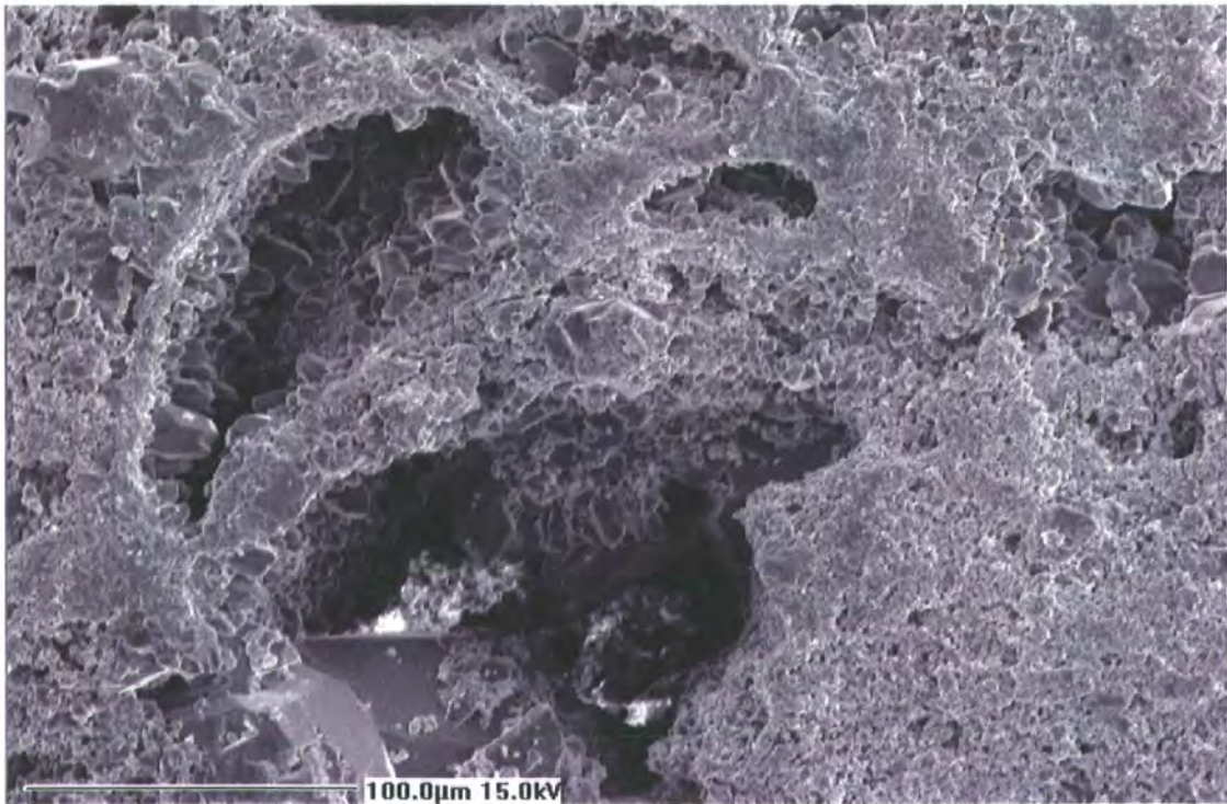
Figure 5.6. SEM Photomicrograph shows partial infill of fully dissolved bioclast by drusy/blocky calcite cement and left mouldic porosity. Jdeir Formation, E1-NC41, 8420.0 feet.
