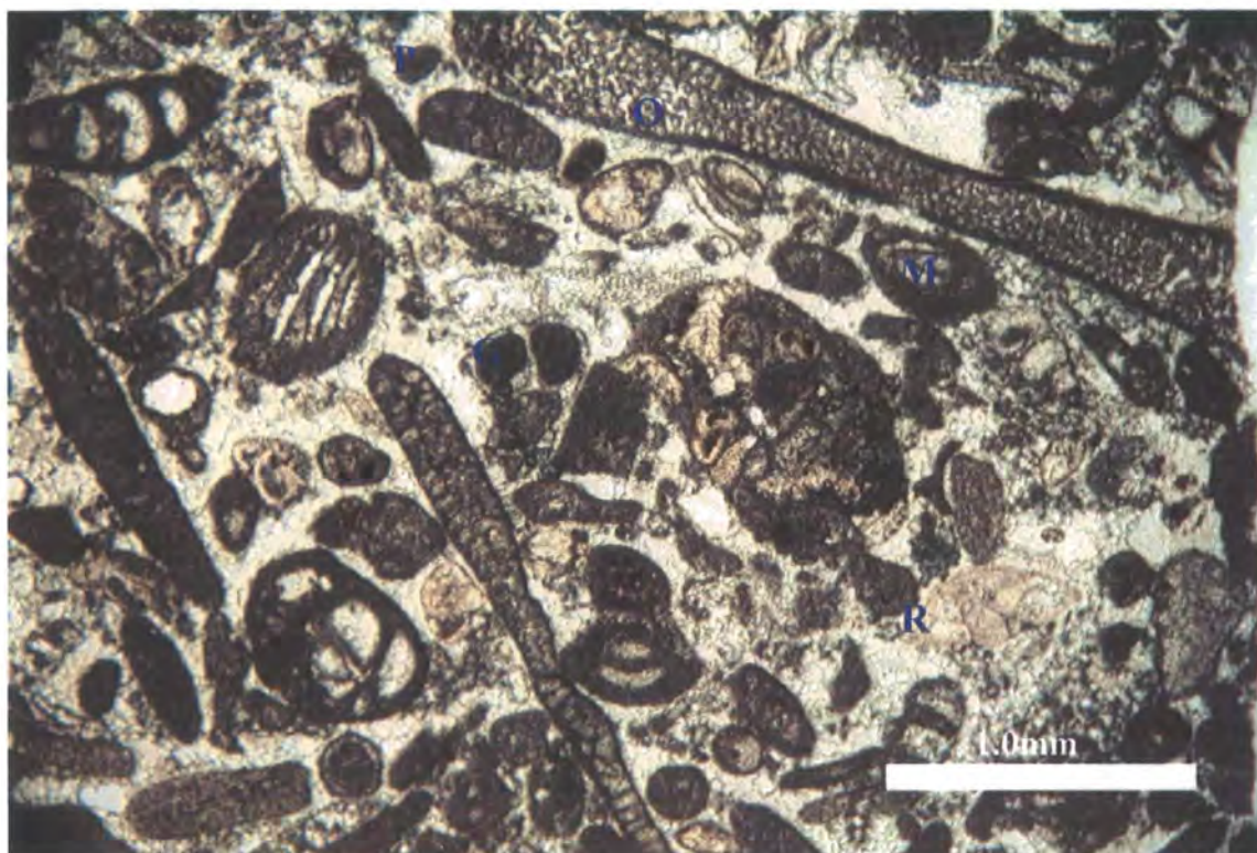
Figure 4.11. Photomicrograph of Alveolina-Orbitolite packstone microfacies containing a mixture of grains include orbitolites (O), miliolid (M), rotaliids (R), small gastropods (G) and peloids (P). Jdeir Formation, E1-NC41 well, 8564.0 feet, PPL.
