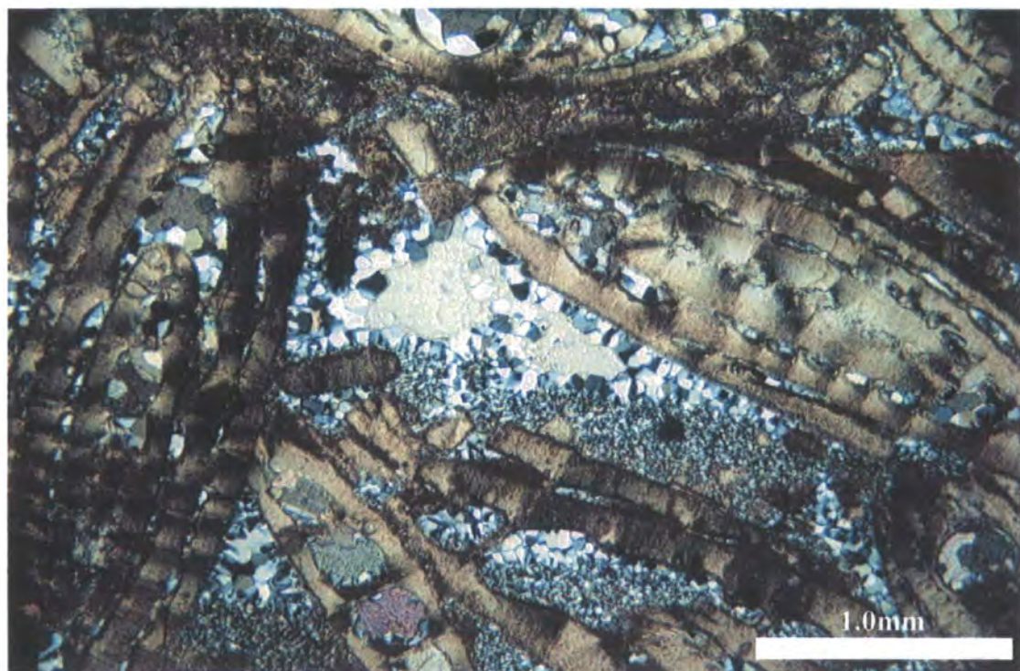
Figure 5.24. Photomicrograph shows silica has completely filled porosity and may have replaced calcite cements. Jdeir Formation, A2-NC41 well, 9262.5 feet, XN.
