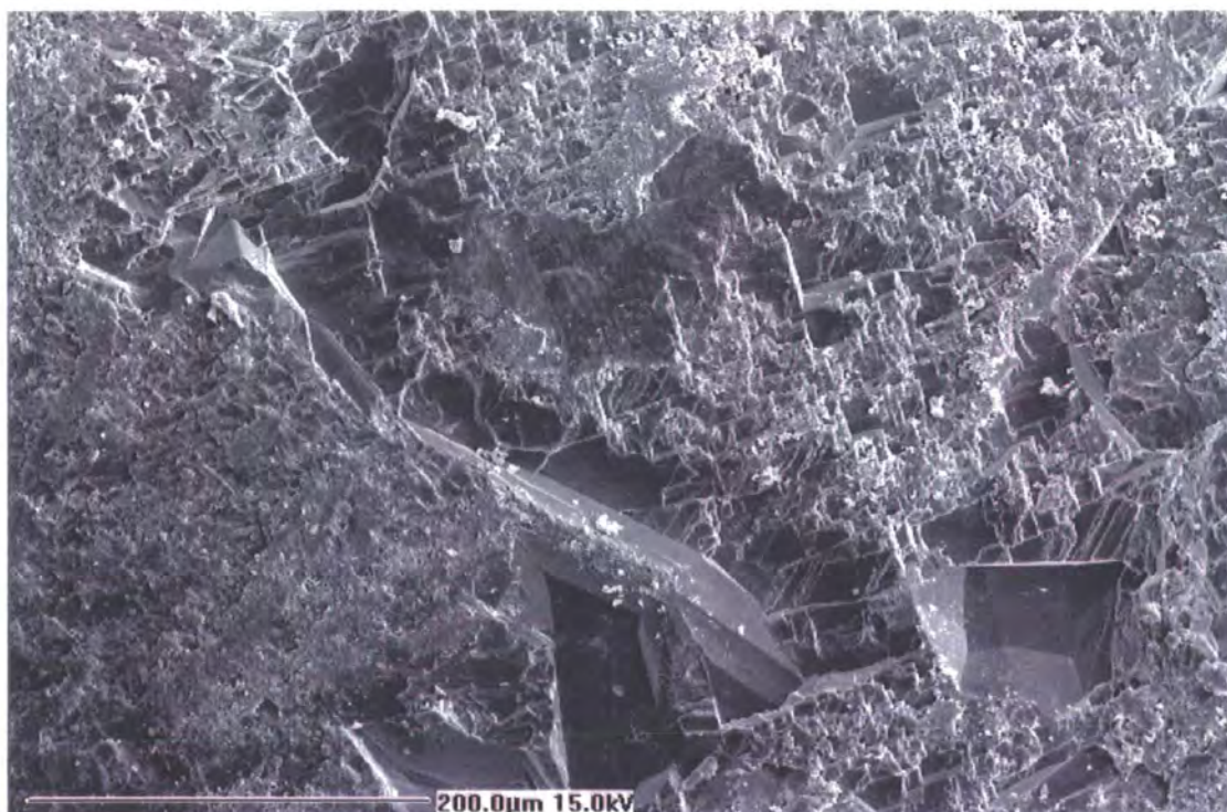
Figure 5.13. SEM Photomicrograph shows blocky calcite cement has completely filled fracture porosity. Jdeir Formation, B7-NC41, 8513.5 feet.
