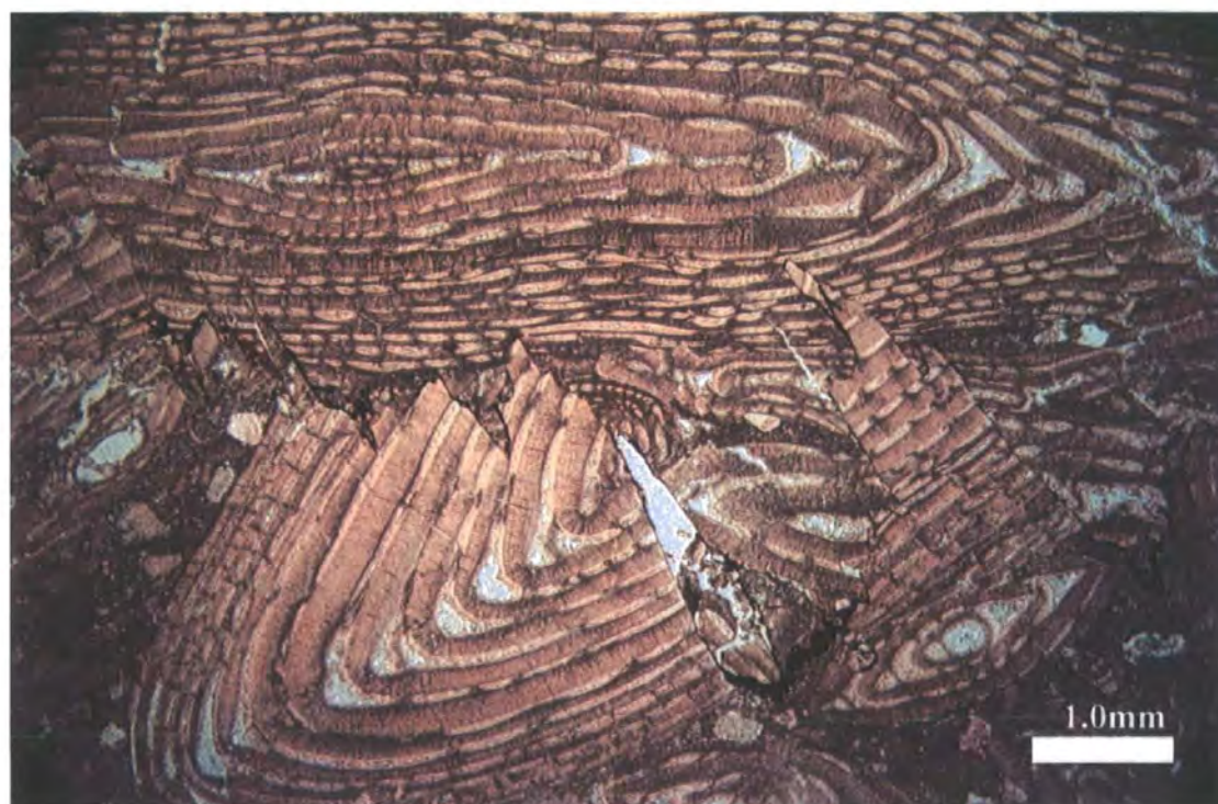
Figure 5.17. Photomicrograph shows nummulites cut by rectangular or high amplitude stylolite. Jdeir Formation, B7-NC41 well, 8460.0 feet, PPL.
