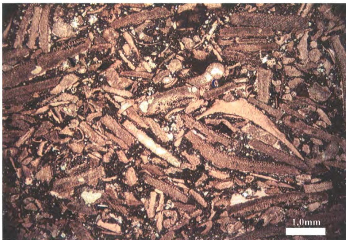
Figure 4.19. Photomicrograph of echinoderm wackestone microfacies dominated by fine to medium, moderately sorted echinoid and crinoid (C) fragments. Jdeir Formation A2-NC41 well, 9249.0 feet, PPL.
