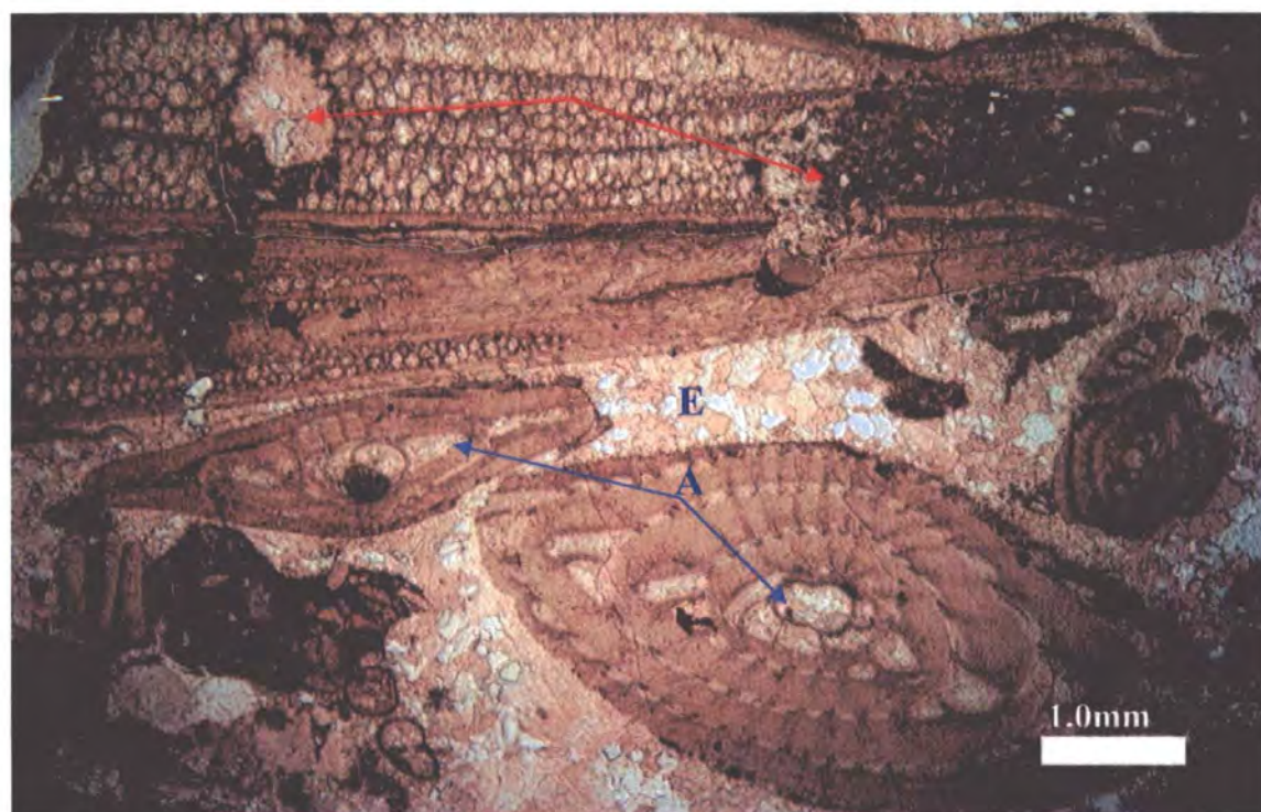
Figure 4.7. Photomicrograph of Nummulite packstone-grainstone/rudstone microfacies with bored mollusc fragment (oyster) (red arrows) and robust nummulite grainstone. Intergranular (E) and intragranular (A) porosity have been completely filled by sparry calcite cement. Jdeir Formation, B7-NC41 well, 8253.0 feet, PPL.
