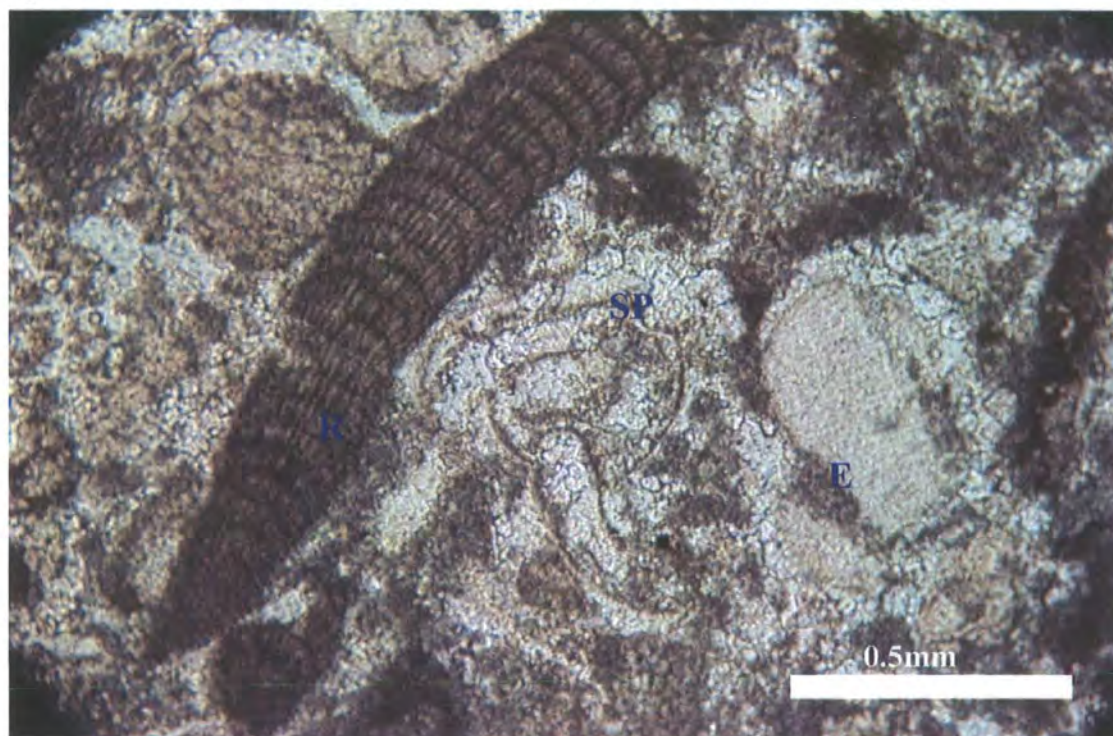
Figure 4.9. Photomicrograph of Alveolina-Molluscan wackestone/packstone microfacies shows a variety of bioclastic grains including Alveolina (A), dasycladacean algae (G), miliolid (M), and bivalves (V) and echinoid fragment (E). Bivalves have been completely dissolved and replaced by equant and drusy calcite cements. Jdeir Formation, E1-NC41 well, 8389.0 feet, PPL.
