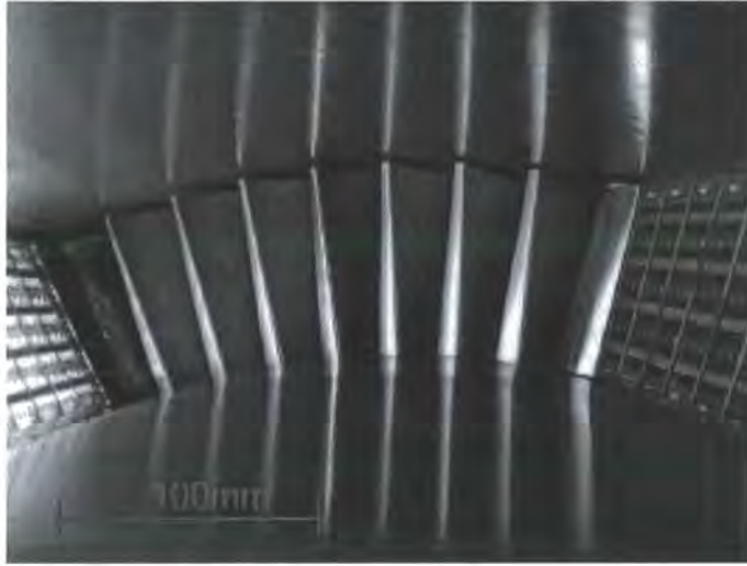
Figure 2.1: Vogt and Fransson's annular sector cascade
