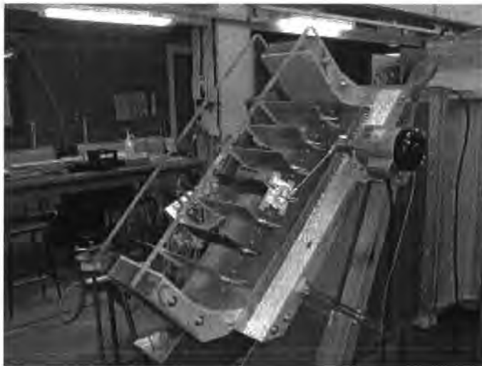
Figure 2.3: Yang and He's compressor cascade
