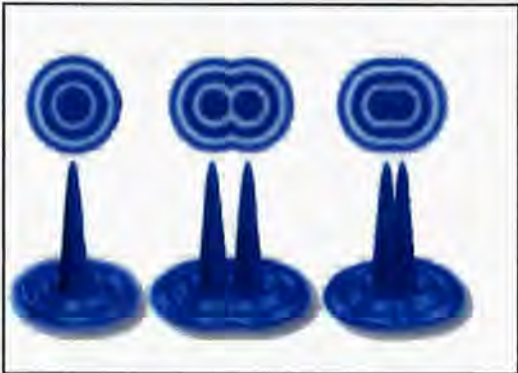
Figure 1: As two point sources of equal intensity approach, they can be resolved at distance up to the resolution limit, which occurs when the central maximum of one Airy Disc coincides with the first minimum of the other. [2]
