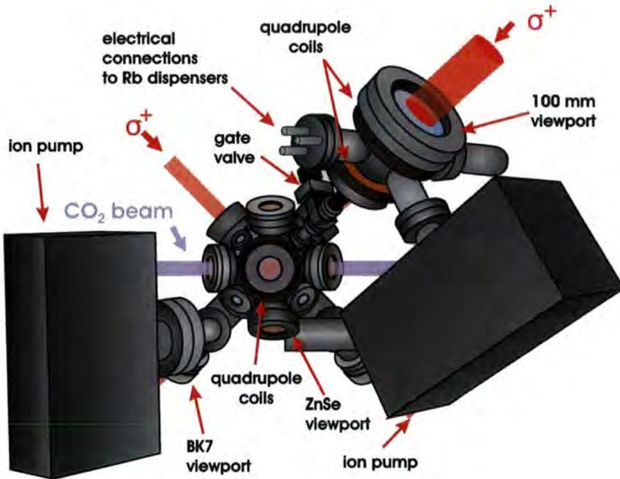
Figure 4.11: Schematic of the double vacuum chamber as viewed from above. All relevant vacuum components are highlighted. Laser beams for the MOTs are shown in red (labeled  $\sigma^\pm$ ) and CO<sub>2</sub> laser trap beams in purple. The quadrupole coils shown on the science chamber are discussed in chapter 6.
