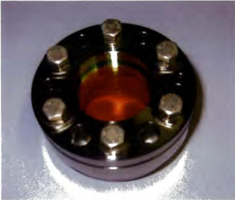
Figure 4.7: Photograph of a home-made vacuum viewport containing a ZnSe window.
