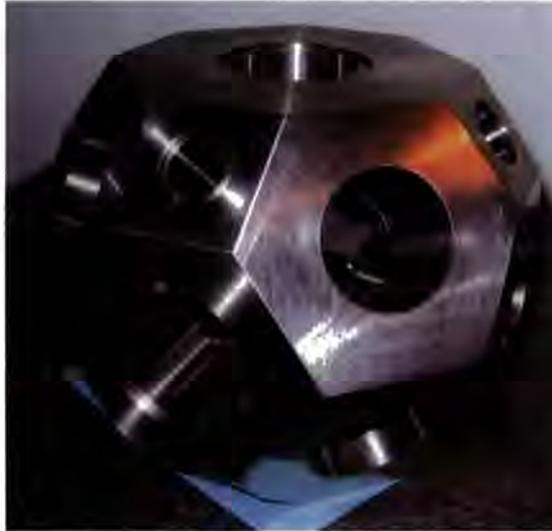
Figure 4.2: Science chamber partially made.
