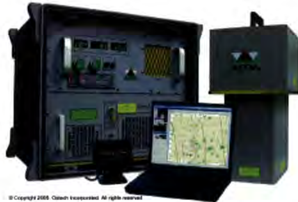
Figure 2.3 The Optech ALTM 3033 laser scanner and associated data collection equipment.
