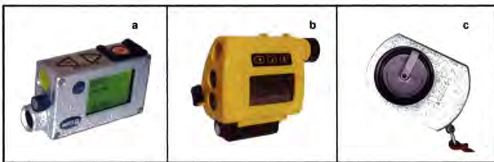
Figure 3.4 The three height measuring devices: (a) Vertex III Hypsometer, (b) LaserAce Hypsometer and (c) Suunto Clinometer.
