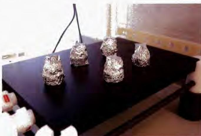
**Fig. 3.7** Rocket vials on the hotplate, with aluminium foil wrapped around the base and the sides. The foil directs the heat up towards the cooler exposed tips of the cone.
