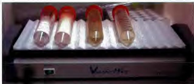
**Fig. 3.4** Shows the 50 mL centrifuge tubes containing the aqua regia, MQ H<sub>2</sub>O and the CCl<sub>4</sub>, on the shaker.
