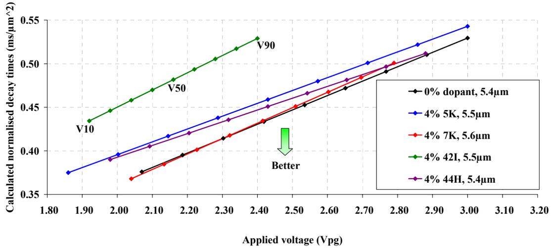
The following experiments were performed using 5μm VA polyimide lined cells at 35 °C, with a 250Hz square wave.
