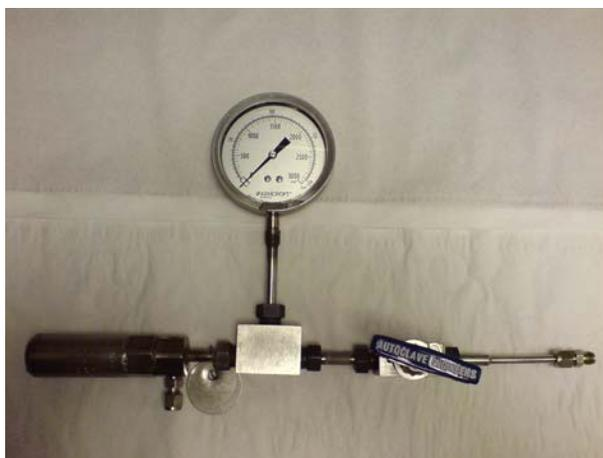
**Figure 17.** Autoclave vessel (25cm<sup>3</sup>) used for high pressure reductions of alkenes
