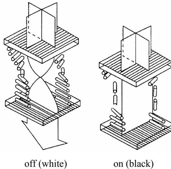
**Figure 2.**<sup>1</sup> Schematic representation of a TN cell
