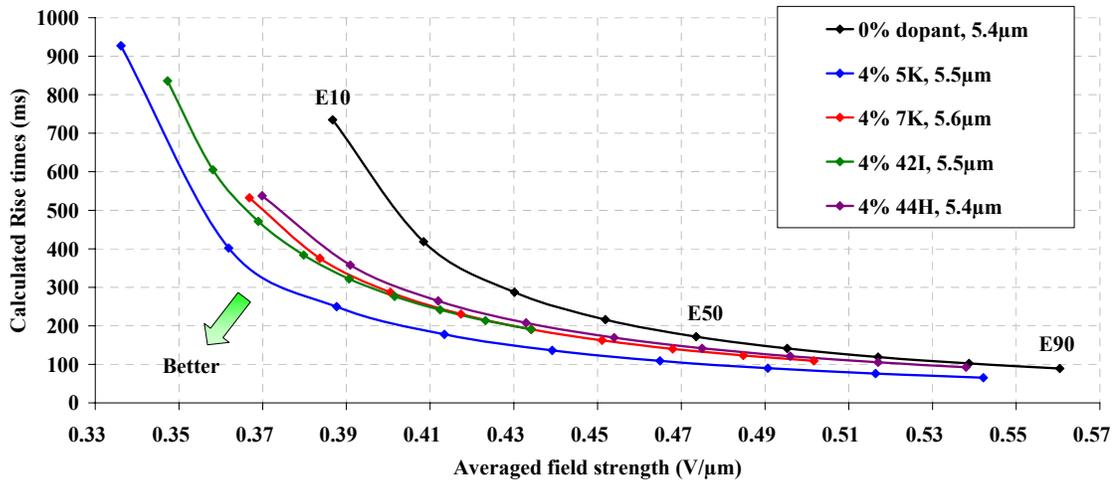
The following experiments were performed using 5 $\mu\text{m}$  VA polyimide lined cells at 35 $^{\circ}\text{C}$ , with a 250Hz square wave.
