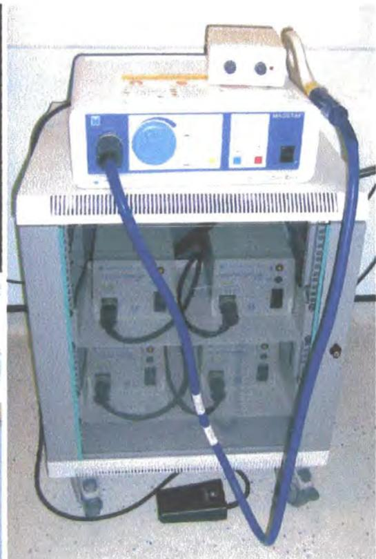
**Figure 1.5b:** Magstim model 200. Trigger pulses from the coil initiate brief magnetic pulses
