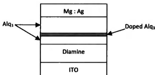
Figure 10 – Device structure reproduced from [18]
