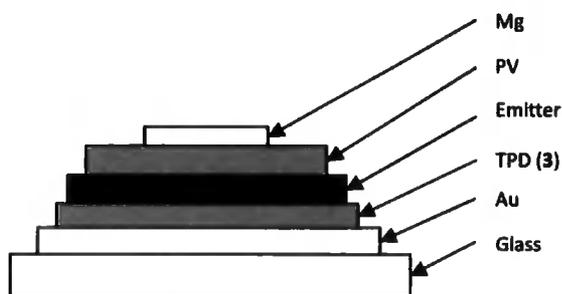
Figure 9 – Device structure reproduced from [10]
