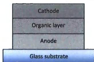
Figure 7 – Schematic diagram of a single layer OLED
