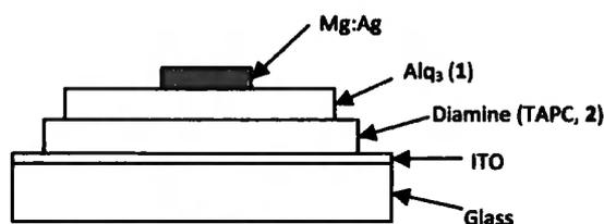
Figure 8 – Device structure reproduced from [8]
