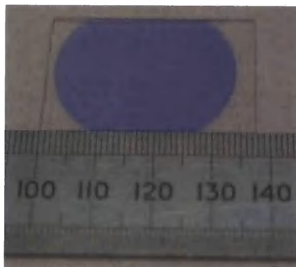
Figure 5.3: Photograph of a 133 nm pentacene thin film on glass slide (38 mm \times 25 mm).
