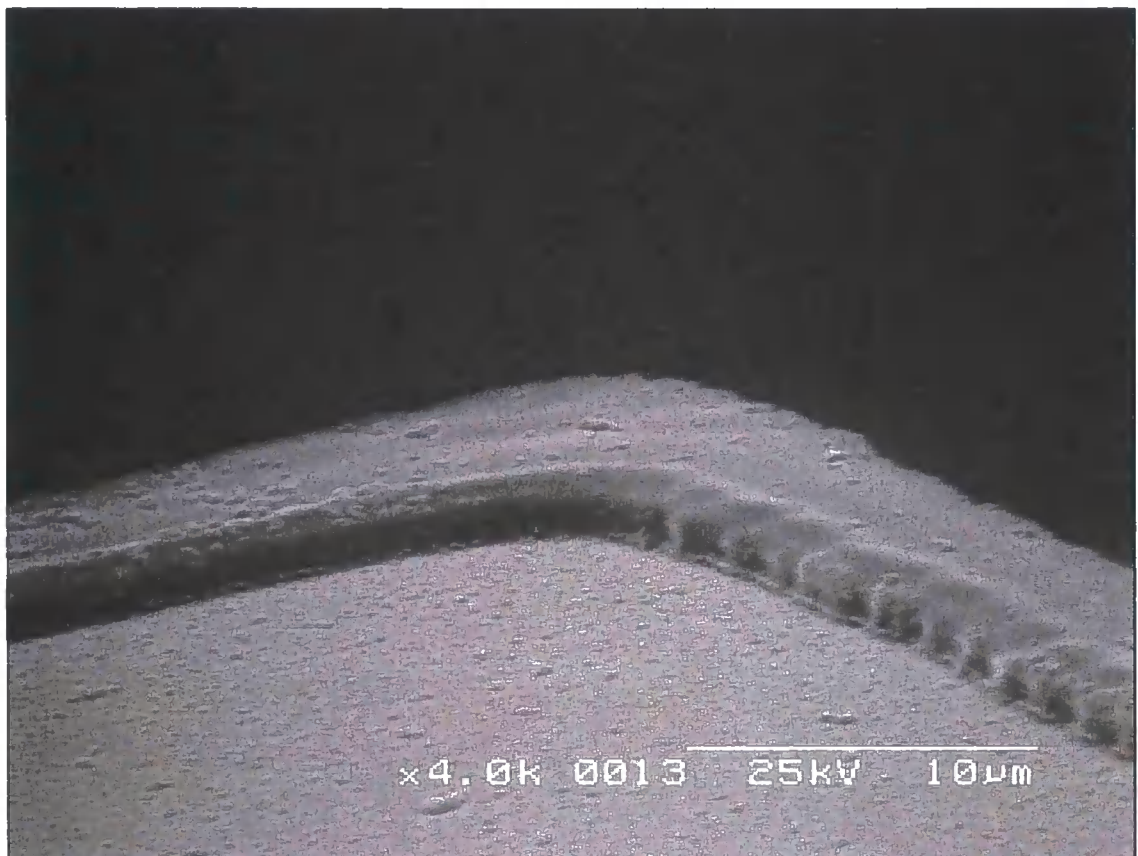
Figure 5-13 Metal contact pads overlapping edges of SU-8
