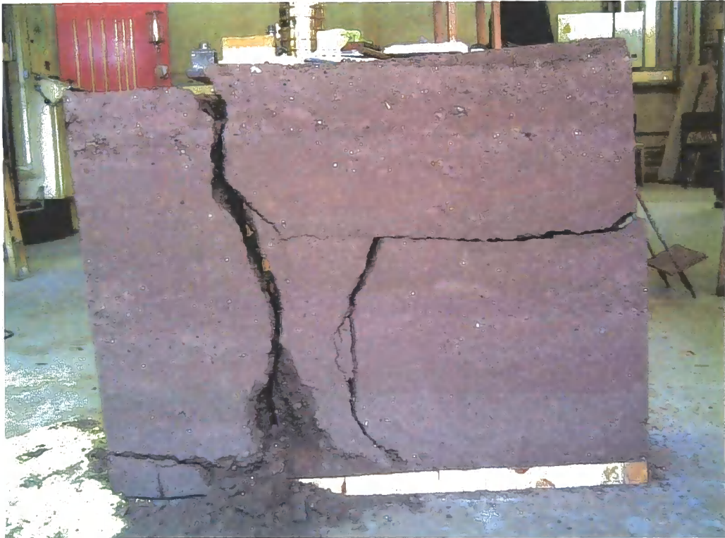
Figure 2.29 Wall 4 loaded and unsupported at left
