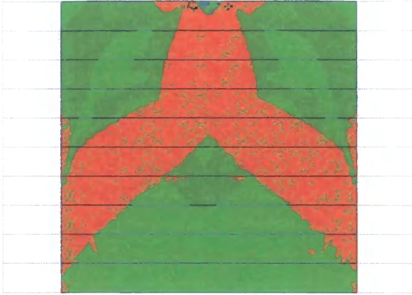
Figure 2.56 Distribution of plastic points on loading of wall. Applied displacement = 12mm. Mohr Coulomb parameters \phi = 35^\circ, c = 75kPa
