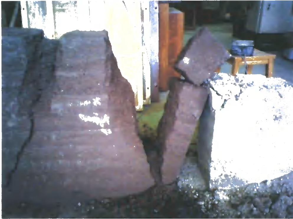
Figure 2.27 Wall 2.3 failure through vertical shear cracking
