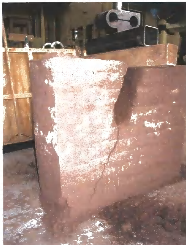
Figure 2.24 Wall 2.2 side A, diagonal shear failure
