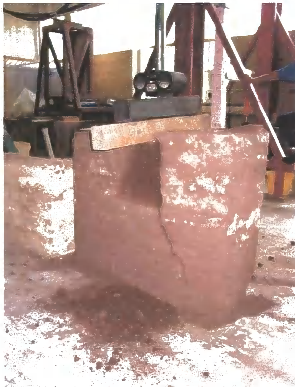
Figure 2.25 Wall 2.2 side B, diagonal shear failure
