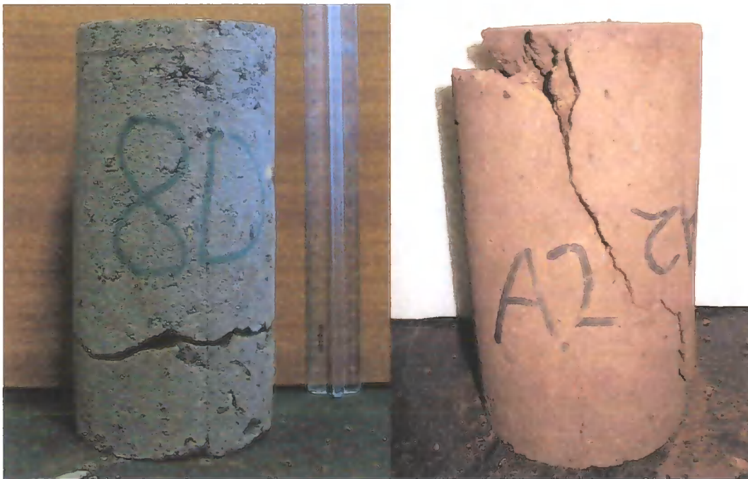
Figure 3.31 Cylinder failure through horizontal delamination (left) and shear (right)
