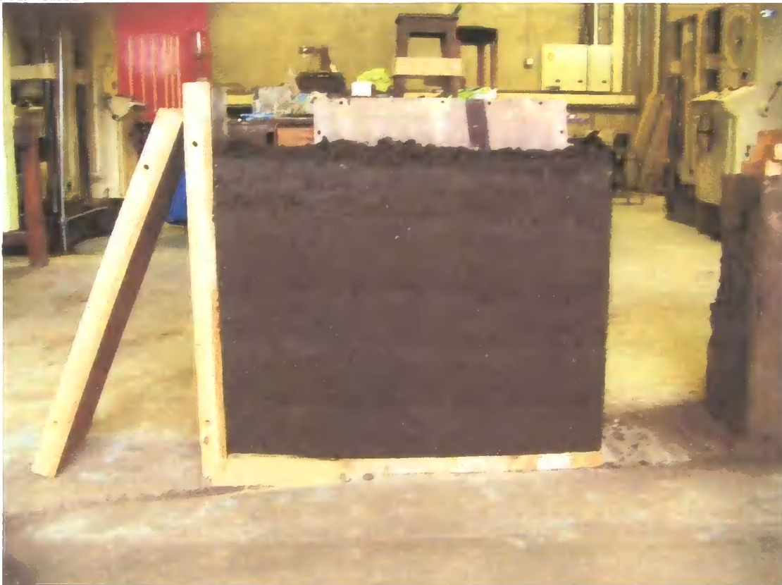
Figure 2.16 Sand and timbers beneath wall 4
