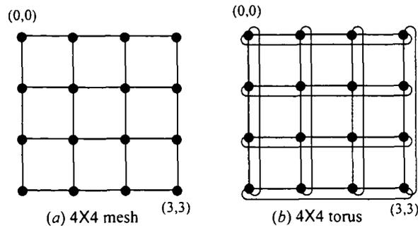
Figure 2.1: Example: (a)  $4 \times 4$  mesh, (b)  $4 \times 4$  torus
