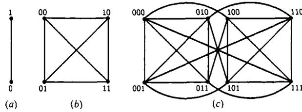
Figure 2.4: Three augmented cubes  $AQ_1$ ,  $AQ_2$  and  $AQ_3$
