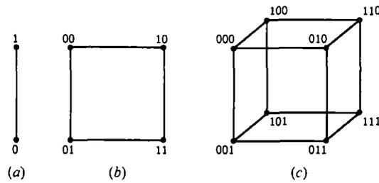
Figure 2.2: Example of hypercubes: (a)  $Q_1$ , (b)  $Q_2$ , (c)  $Q_3$
