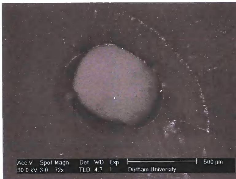
Figure 5.6. SEM image of a 500  $\mu\text{m}$  diameter pinhole on a CdS film, magnification used is 72 times.
