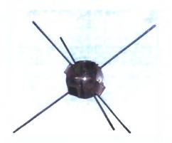
Figure 1.5. The first PV powered satellite Vanguard 1, measuring only 15 cm in diameter and weighing 1.5 kg it had six single crystal silicon PV cells (four are visible in the above image).
