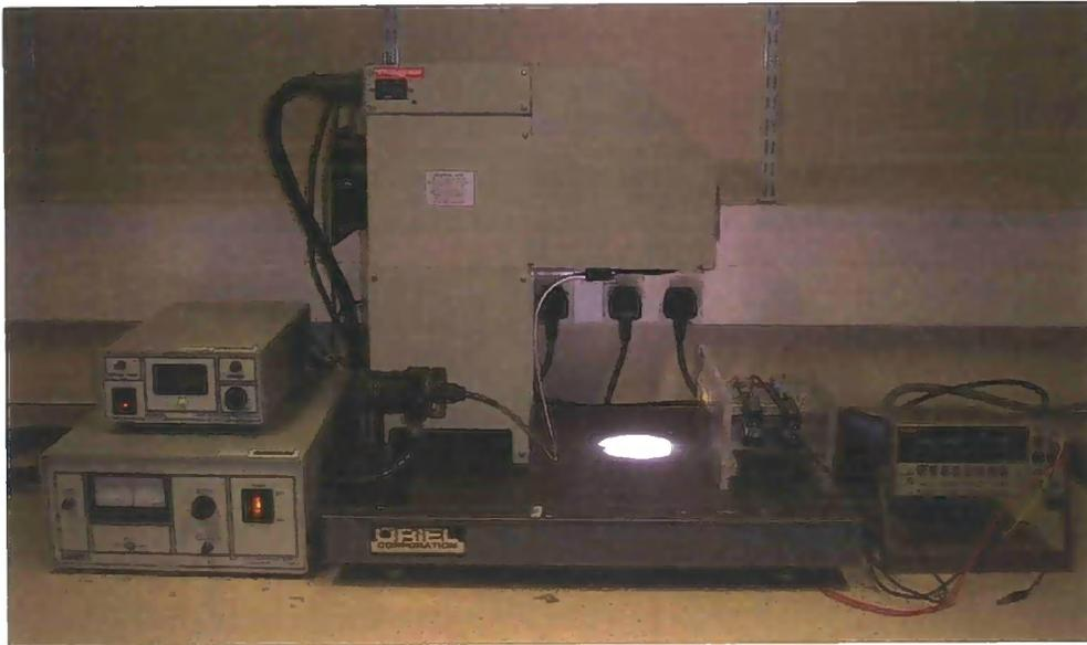
Figure 4.17. Oriel solar simulator, showing power supply and power output indicator (left bottom and top respectively), light output (centre), sample holder (centre-right) and Keithley sourcemeter (right).
