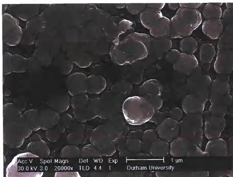
Figure 5.8 SEM image of a CdS film composed of colloidal particles, magnification used is 20k times.
