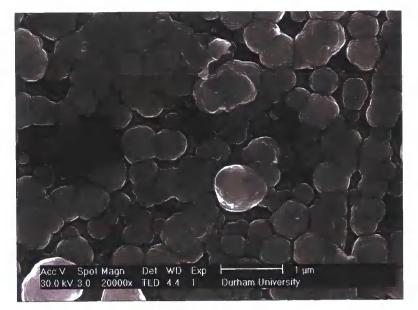
Figure 5.8 SEM image of a CdS film composed of colloidal particles, magnification used is 20k times.
