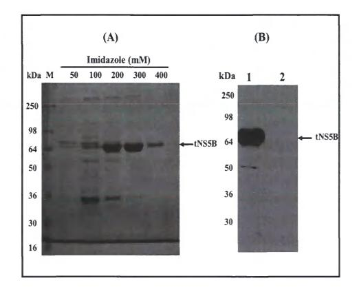
Fig. 4.2: Expression of tNS5B in fusion with His-tag. (A) Overexpression and Purification of tNS5B. tNS5B was expressed in *E. coli* BL21 (DE3) and captured using a HiTrap metal ion chelating column. The protein was eluted with increasing concentrations of imidazole. (B) Detection of tNS5B was performed using α-His-HRP antibody for His-tag. 1- tNS5B purified protein and 2- Total protein extracted from *E. coli* BL21 (DE3) cells transformed by empty pET21d.
