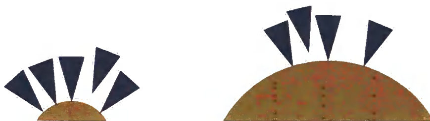
Figure 4.9: Schematic of polymeric ligand packing on the surface of particles of radii 1 and 3. On larger particles, ligands (triangles) pack less densely as the lower curvature of the surface results in increased steric hinderance in the corona.
