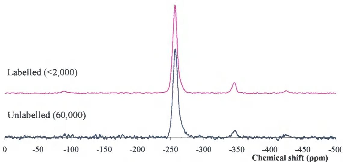
**Figure 5.74 -  $^{15}\text{N}$  CPMAS ssNMR of purified samples of chitin extracted from *M. rouxii* cultured in labelled (containing  $(^{15}\text{NH}_4)_2\text{SO}_4$ ) and unlabelled media. The number of repetitions required to obtain the spectra are shown in brackets.**
