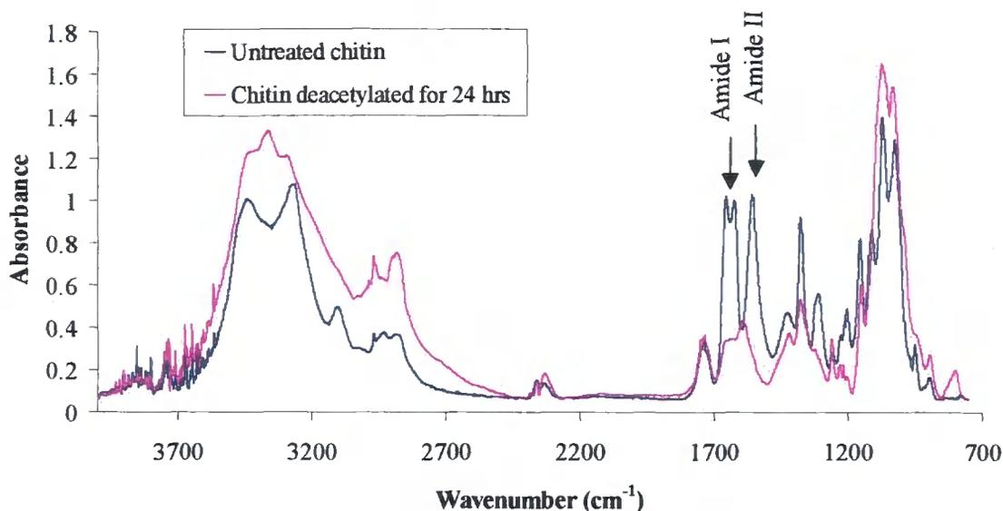
**Figure 3.8 - IR spectra of commercial chitin, untreated and deacetylated in 40 % NaOH at 100 °C under nitrogen for 24 hours.**
