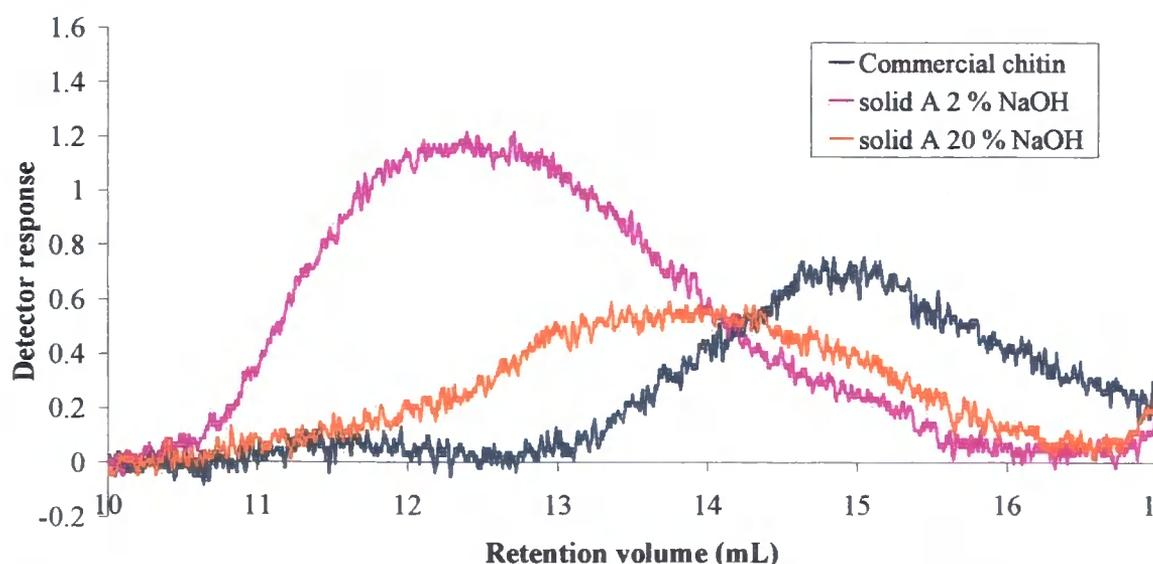
**Figure 4.38 – Refractive index trace produced by GPC analysis of a commercial sample of chitin (Sigma) and two samples of solid A extracted by chemical extraction procedure two using varying concentrations of NaOH in the deproteinisation step. 5 % (w/v) LiCl:DMAC was used as the solvent and eluent.**
