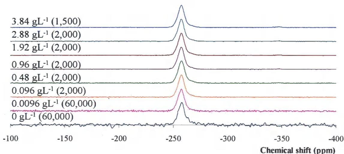
**Figure 5.71** -  $^{15}\text{N}$  CPMAS ssNMR spectra of chitin extracted from fungal biomass cultured in growth media containing varying concentrations of  $(^{15}\text{NH}_4)_2\text{SO}_4$ . The number of repetitions required to obtain the spectra are shown in brackets.
