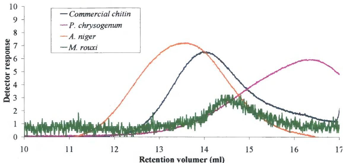
**Figure 4.62 - Refractive index trace produced by the GPC analysis of commercial chitin (Sigma), the purified solid A extracts from 'wet' *P. chrysogenum*, *A. niger* and *M. rouxii* biomass using 5 % (w/v) LiCl:DMAc as the solvent and eluent.**
