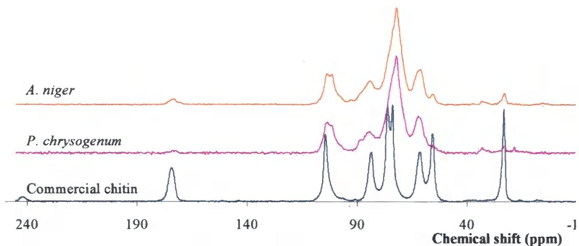
Figure 4.57 -  $^{13}\text{C}$  CPMAS ssNMR spectrum of the crude materials obtained from the enzymatic extraction of 'wet' *A. niger* and *P. chrysogenum* biomass. A commercial source of chitin (Sigma) is shown for comparison.
