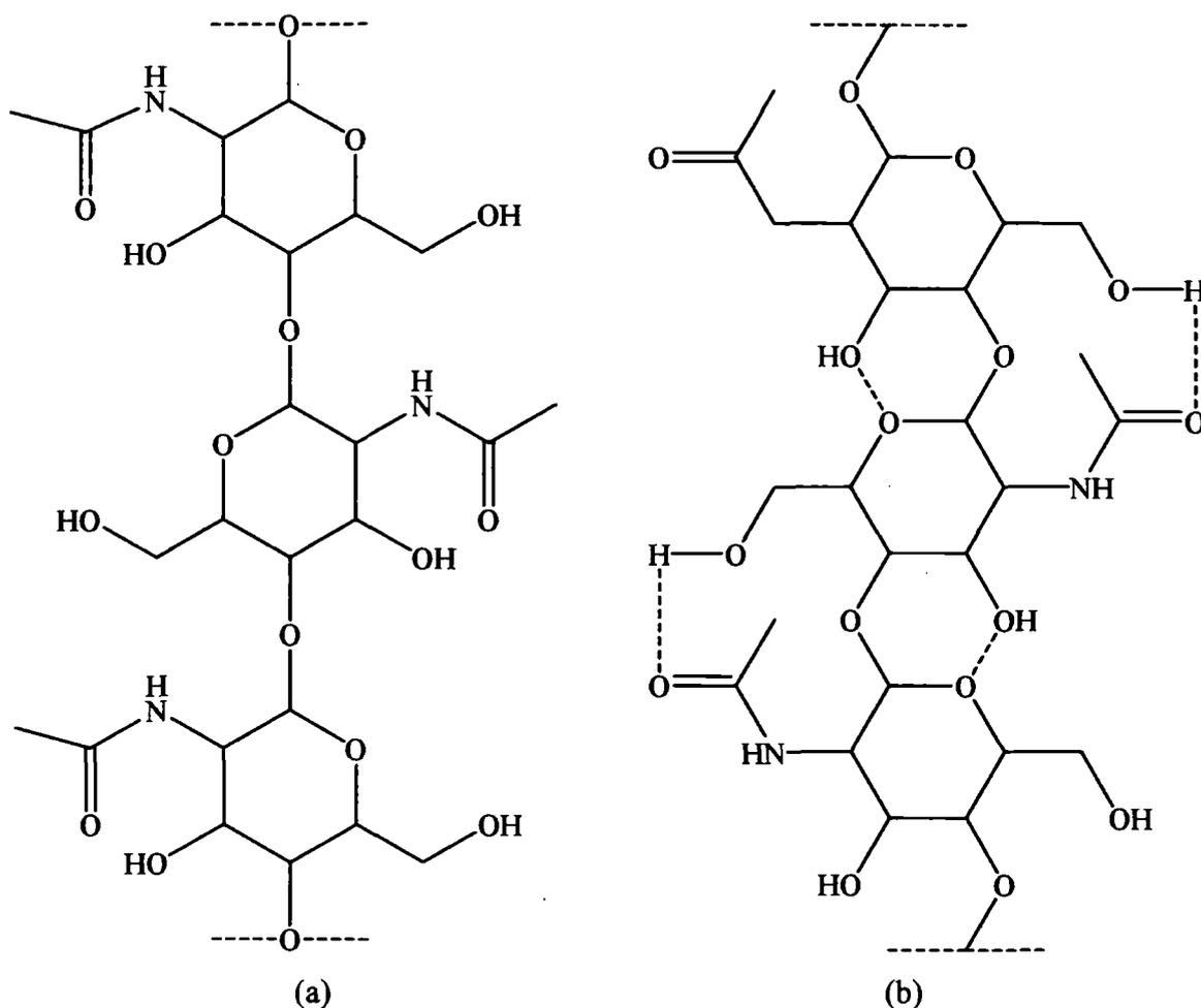
**Figure 1.3 - Straight (a) and bent (b) conformations of the repeat disaccharide unit in the chitin chain.**
