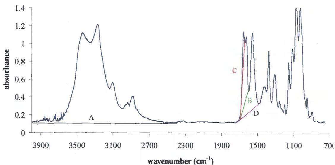
**Figure 3.7 - FTIR spectrum of a commercial sample of chitin. The proposed baselines used to calculate the absorption of the bands at, A -  $3450\text{ cm}^{-1}$ , B -  $1655\text{ cm}^{-1}$ , C -  $1630\text{ cm}^{-1}$  and D -  $1655\text{ cm}^{-1}$  are marked.**
