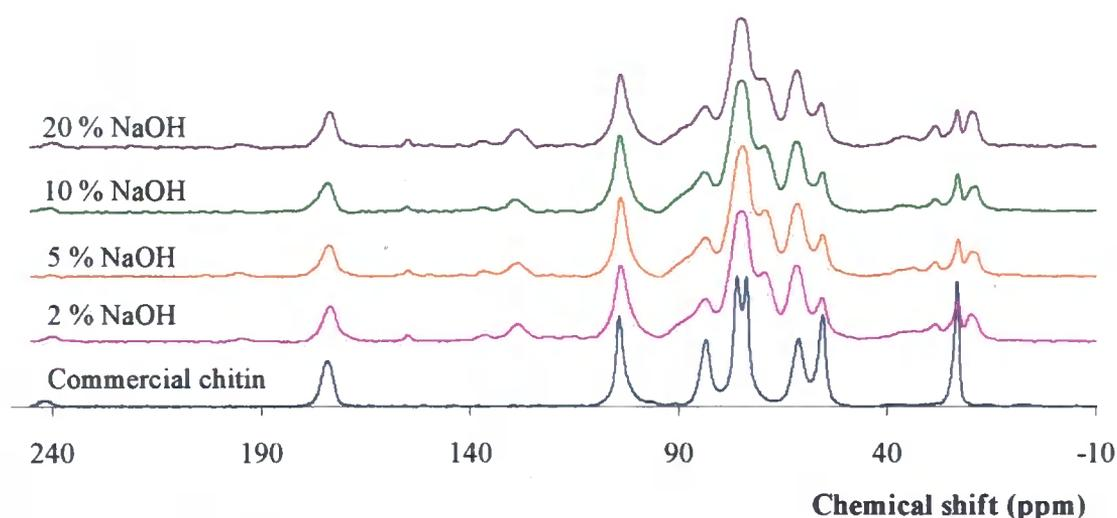
**Figure 4.37 -  $^{13}\text{C}$  CPMAS ssNMR spectra of commercial chitin and a series of samples of solid A, containing crude chitin, extracted by chemical extraction procedure two using varying concentrations of NaOH in the deproteinisation step.**
