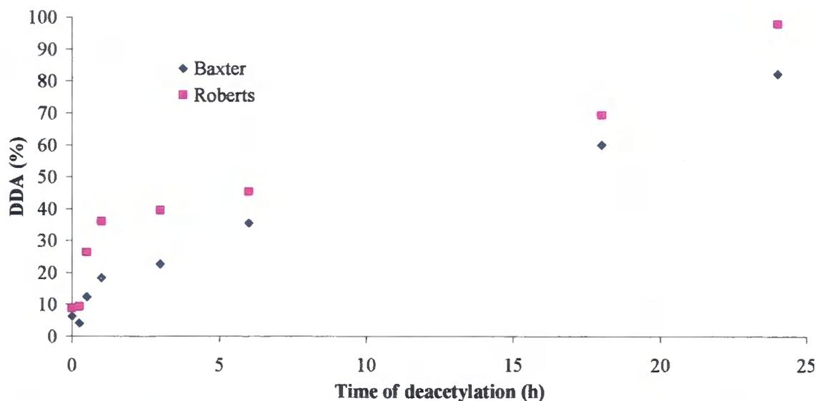
**Graph 3.4 - The DDA of a series of samples of commercial chitin deacetylated for varying lengths of time. DDA is determined from the ratio of the absorbance of the amide I band to the OH stretching band at  $3450\text{ cm}^{-1}$  using the methods of Baxter[158] and Roberts.[159]**
