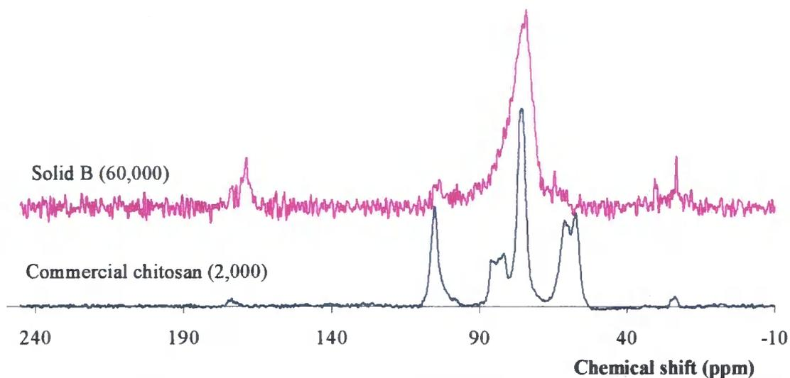
**Figure 4.35 -  $^{13}\text{C}$  CPMAS ssNMR spectra of solid B extracted by chemical extraction procedure two,[103] and commercial chitosan (Sigma) The number of repetitions required to obtain the spectra are shown in brackets.**
