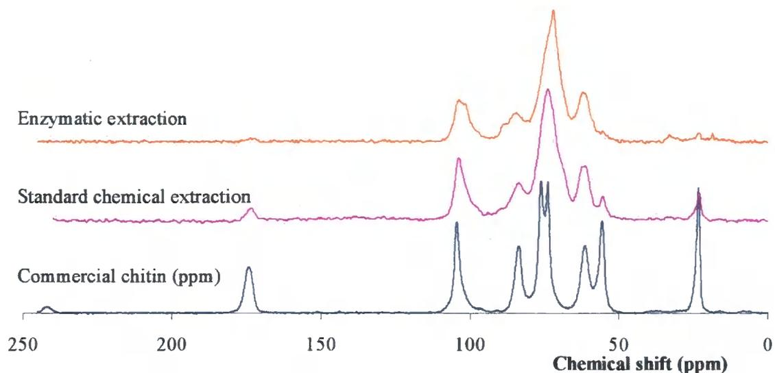
**Figure 4.56 -  $^{13}\text{C}$  CPMAS ssNMR spectra of crude chitin samples extracted from 'wet' *P. chrysogenum* by the standard chemical procedure and by the enzymatic procedure of Cai *et al.*[102]**
