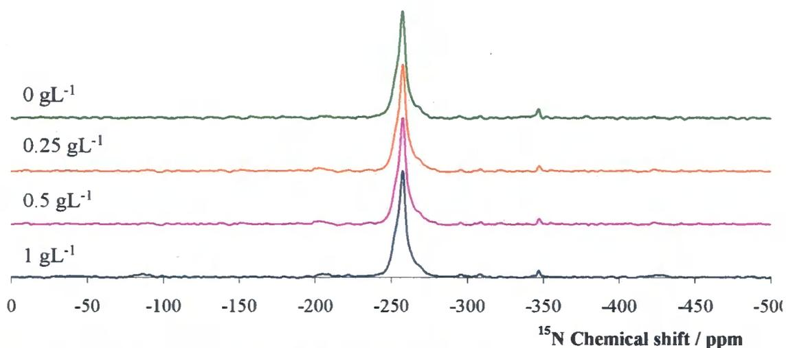
**Figure 5.72** -  $^{15}\text{N}$  CPMAS ssNMR spectra of sterilised 'whole cell' samples of *P. chrysogenum* cultured in modified medium A (rich) containing varying concentrations of peptone, concentration shown above each spectra. 2,000 repetitions were required to acquire the spectra.
