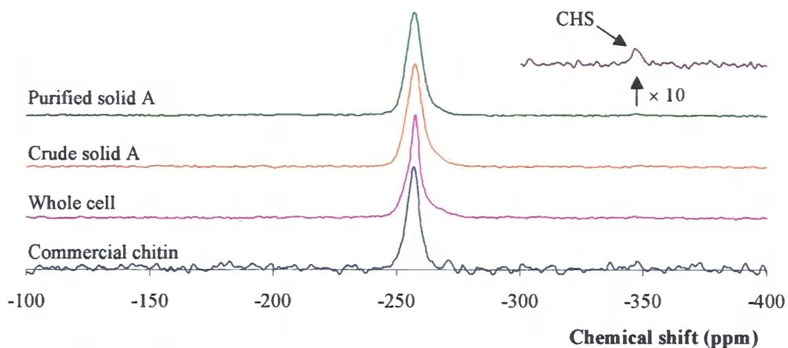
**Figure 4.47** -  $^{15}\text{N}$  CPMAS ssNMR spectra of the whole cell sample of *P. chrysogenum*, the crude chitin containing fraction, solid A, and the purified chitin fraction. The spectrum of a commercial sample of chitin (Sigma) is shown for comparison. The chemical shift range of purified solid A between  $-300$  to  $-400$  ppm is expanded ( $\times 10$ ). CHS = amino peak of chitosan.
