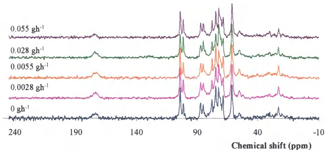
**Figure 6.78 -  $^{13}\text{C}$  CPMAS ssNMR spectra of whole 'wet' samples of biomass cultured with the addition of PAA at varying feeding rates**
