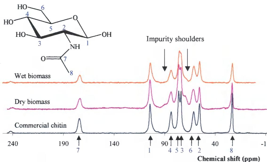
**Figure 4.49 - <sup>13</sup>C CPMAS ssNMR spectra of purified chitin extracted from the dry biomass obtained from Angel Biotechnology and from wet biomass produced by the incubation of *P. chrysogenum*. The spectrum of a commercial sample of chitin (Sigma) is shown for comparison.**
