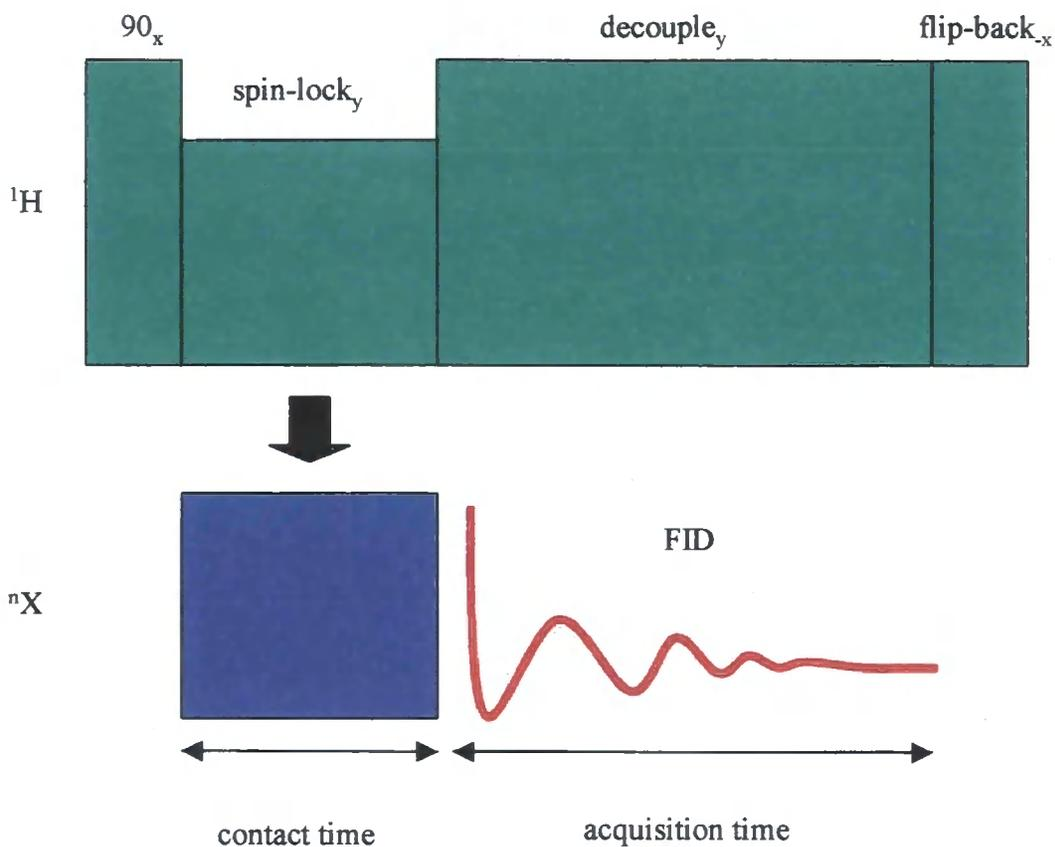
**Figure 3.22 - Pulse sequence employed to obtain a ssNMR spectrum using the cross-polarisation technique.**
