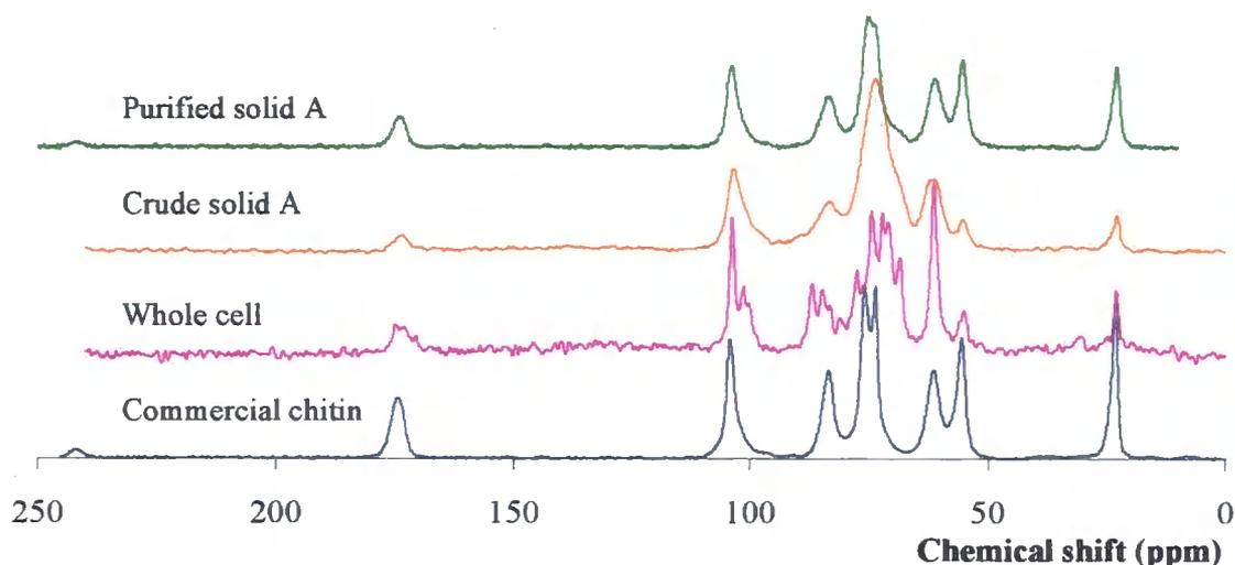
**Figure 4.46 -  $^{13}\text{C}$  CPMAS ssNMR spectra of the whole cell sample of *P. chrysogenum*, the crude chitin containing fraction, solid A, and the purified chitin fraction. The spectrum of a commercial sample of chitin (Sigma) is shown for comparison.**
