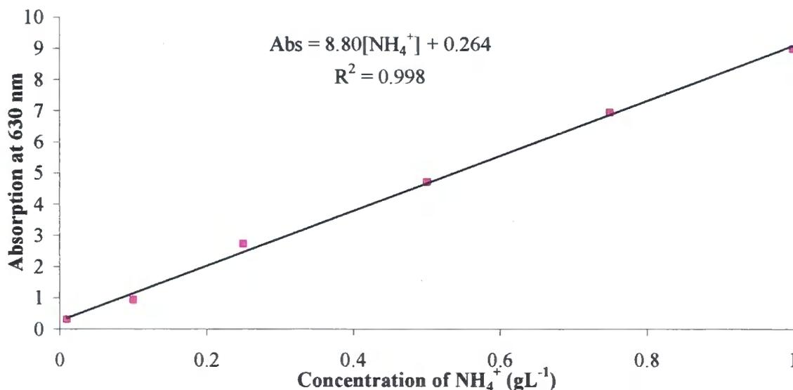
Graph E.17 - Standardisation of the NH<sub>4</sub><sup>+</sup> assay using known concentrations of ammonium sulfate
