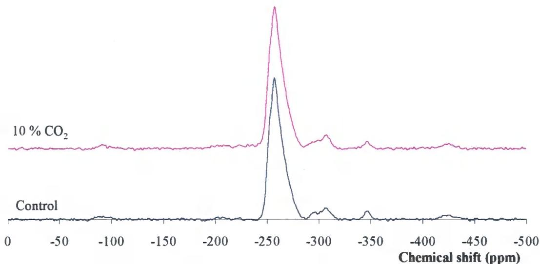
**Figure 6.77 -  $^{15}\text{N}$  CPMAS ssNMR of whole cell samples cultured on agar plates at 24 °C under normal atmospheric conditions and at carbon dioxide concentrations of 10 %.**
