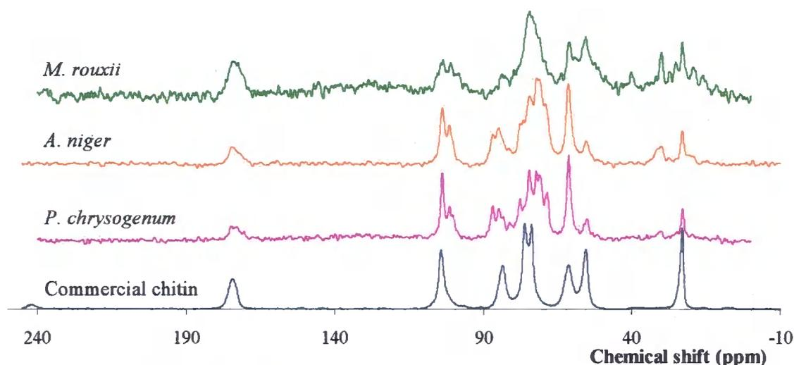
**Figure 4.58** -  $^{13}\text{C}$  CPMAS ssNMR spectra of the whole cell samples of *P. chrysogenum*, *A. niger* and *M. rouxii*. The spectrum of a commercial source of chitin (Sigma) is shown for comparison.
