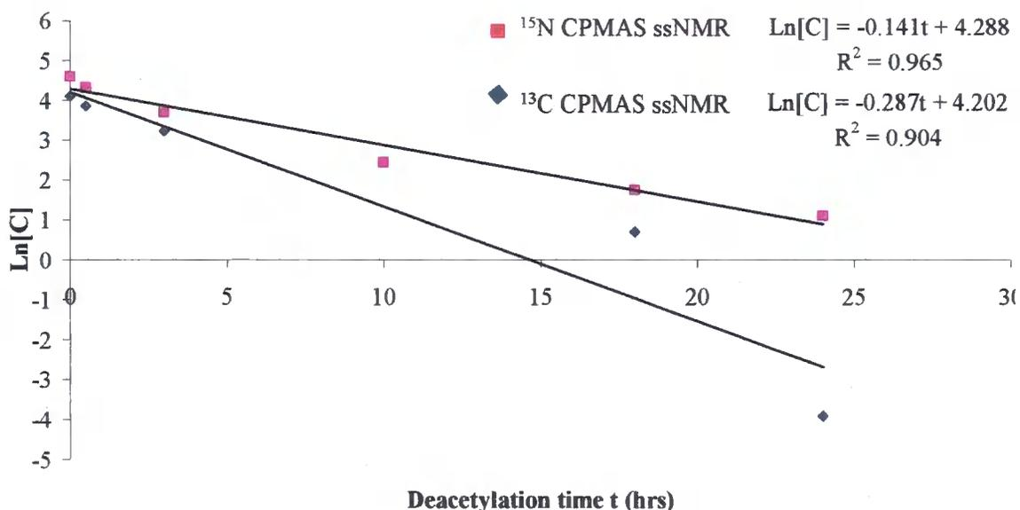
**Graph 5.15 - Pseudo first order rate plot of the deacetylation of chitin in alkali. Where  $[C]$ , the concentration of *N*-acetyl-D-glucosamine, is determined by  $^{15}\text{N}$  and  $^{13}\text{C}$  CPMAS ssNMR**
