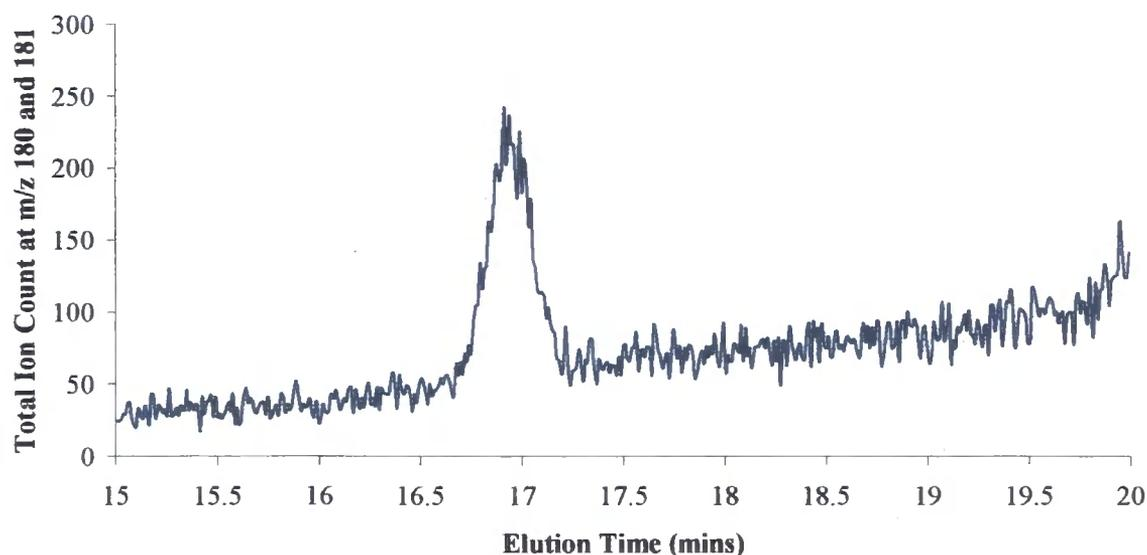
**Graph 5.8 - Chromatogram of hydrolysed chitinous material showing mass ions 180 and 181.**
