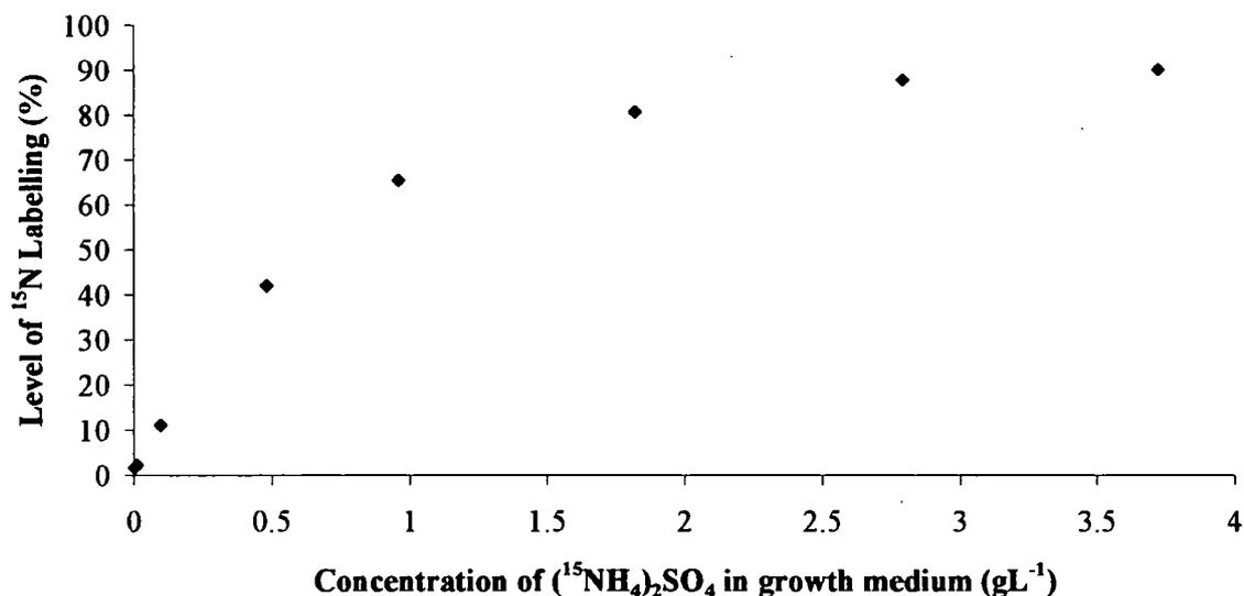
**Graph 5.11 - Level of  $^{15}\text{N}$  labelling in samples cultured in media with varying concentrations of  $(^{15}\text{NH}_4)_2\text{SO}_4$  calculated from the average relative intensity of the 163.1 and 181.1 mass ion peaks in the isotopic distribution about the mass ion at  $m/z$  162.1 and 180.1 respectively.**
