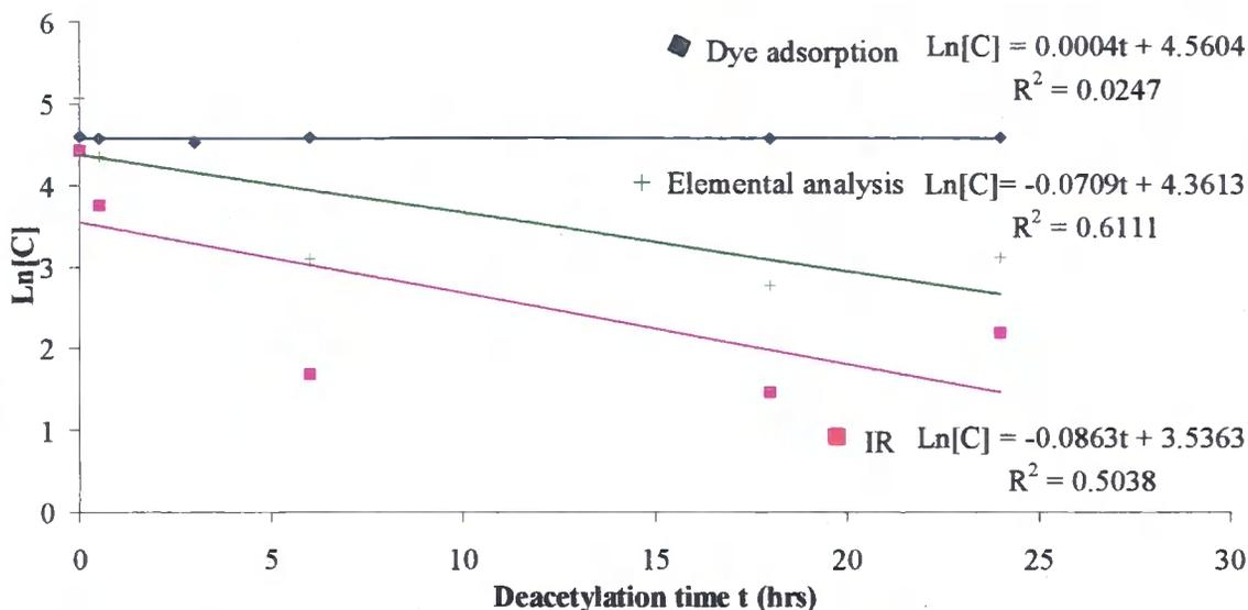
**Graph 5.16 - Pseudo first order rate plot of the deacetylation of chitin in alkali. Where [C], the concentration of *N*-acetyl-D-glucosamine, is determined by the dye adsorption method, IR spectroscopy and elemental analysis.**
