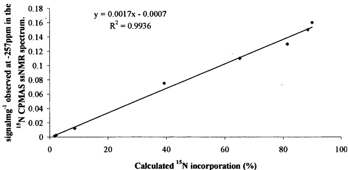
**Graph 5.13 - Amount of signal per milligram of sample seen at  $\sim -257$  ppm (corresponding to chitin) in the  $^{15}\text{N}$  CPMAS ssNMR spectra of samples against the calculated degree of  $^{15}\text{N}$  labelling.**
