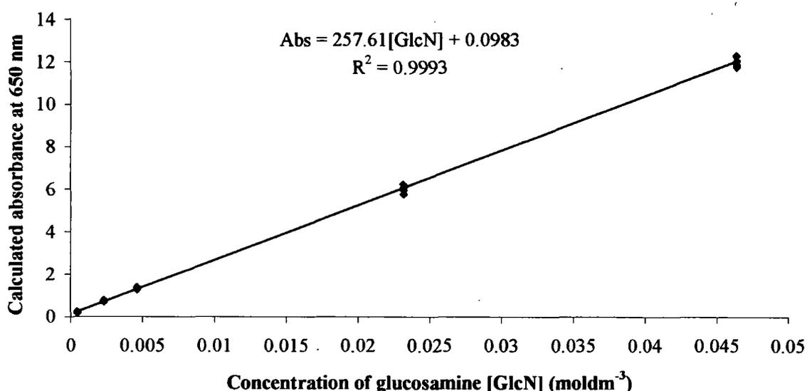
**Graph 3.1 – Standard plot of glucosamine concentration against absorbance at 650 nm following the assay proposed by Tsuji et al.[131]**
