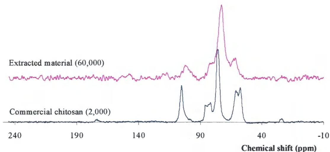
**Figure 4.31 -  $^{13}\text{C}$  CPMAS ssNMR spectra of commercial chitosan (Sigma) and a sample of material extracted by chemical extraction procedure 1.[115] Number of repetitions to acquire the spectra shown in brackets.**
