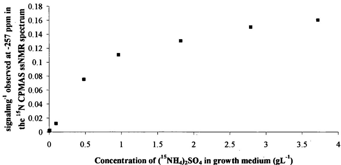
**Graph 5.12 – Amount of signal seen at  $\sim 257$  ppm, corresponding to chitin, per milligram of sample in the  $^{15}\text{N}$  CPMAS ssNMR spectra of chitinous extracts of materials cultured in growth media of varying concentrations of  $(^{15}\text{NH}_4)_2\text{SO}_4$ .**
