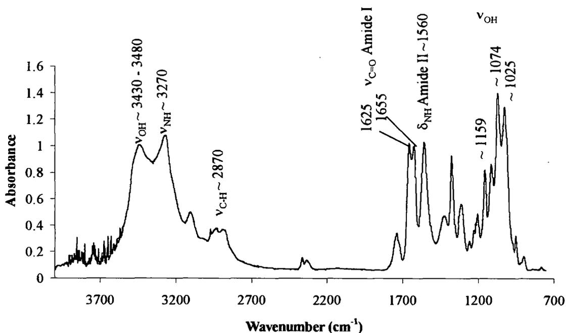
**Figure 3.6 - FTIR spectrum of a commercial sample of chitin (Sigma) obtained in absorbance mode. The most commonly used probe and reference absorption bands used in the determination of the DDA in the literature are marked.**
