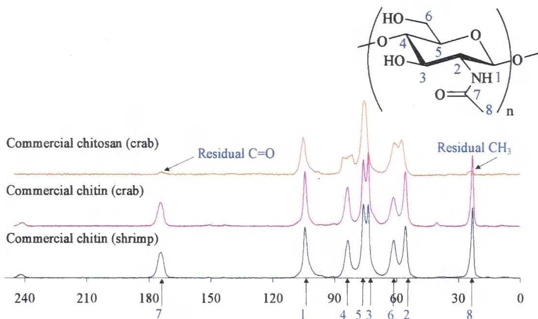
Figure 3.23 -  $^{13}\text{C}$  CPMAS ssNMR of commercial sources of chitin and chitosan supplied by Sigma. The source of the chitinous material is shown in brackets.
