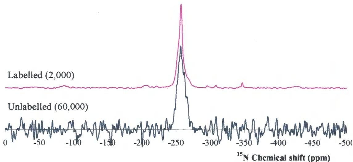
**Figure 5.73 -  $^{15}\text{N}$  CPMAS ssNMR spectra of wet mycelium cultured in labelled and unlabelled media. The number of repetitions required to obtain the spectra are shown in brackets.**
