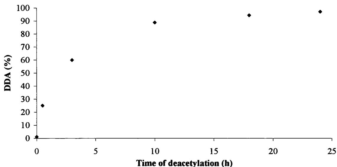
**Graph 5.14 - DDA of a series of samples of chitin extracted from *P. chrysogenum*, cultured in  $^{15}\text{N}$  labelled conditions, deacetylated for varying lengths of time. DDA determined by  $^{15}\text{N}$  CPMAS ssNMR**
