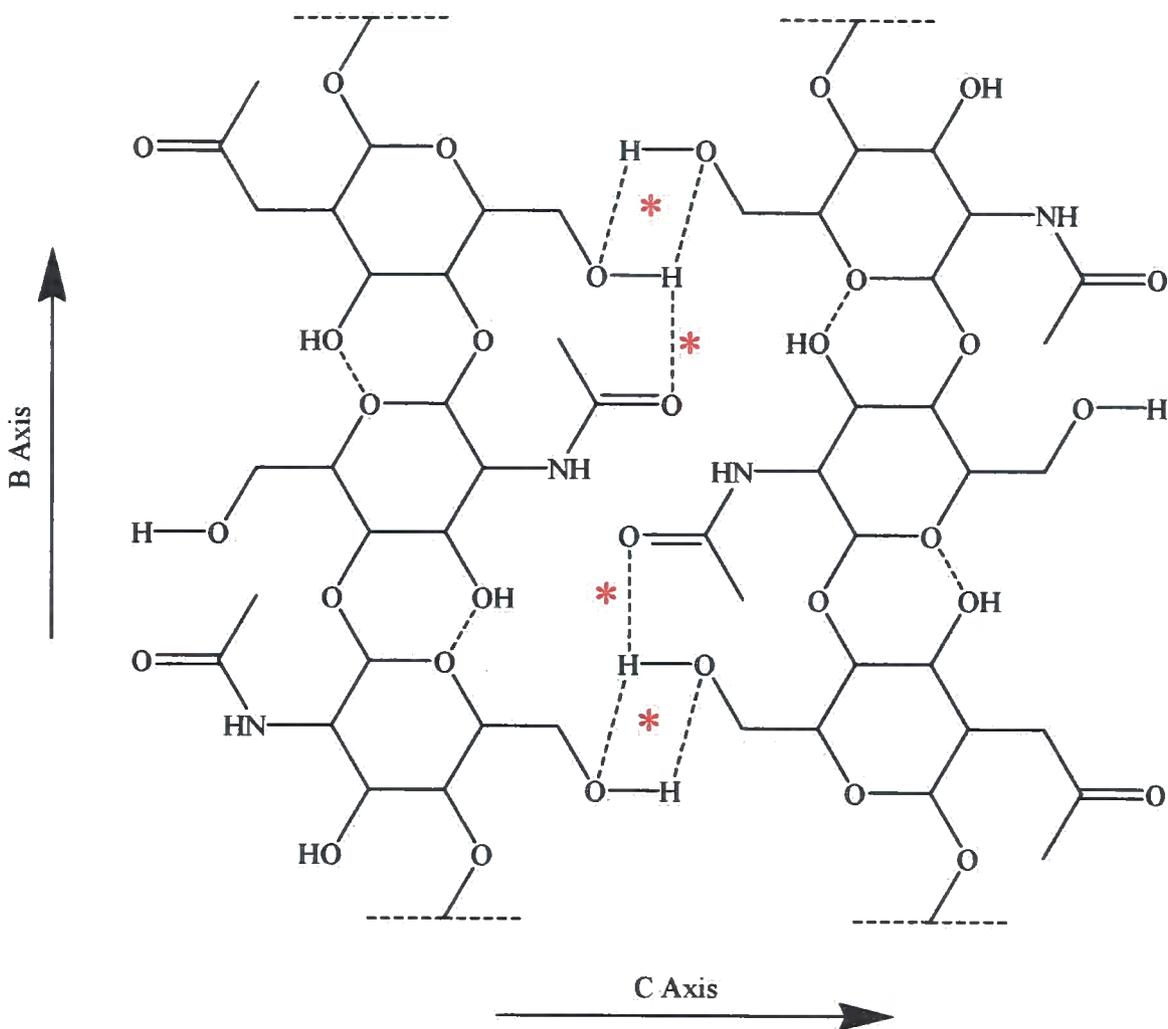
**Figure 1.4 - Intermolecular hydrogen bonding present in  $\alpha$ -chitin (A axis is perpendicular to the plane) Dashed lines represent hydrogen-bonds. \* Represents hydrogen bonds present in a 50:50 statistical mix.**
