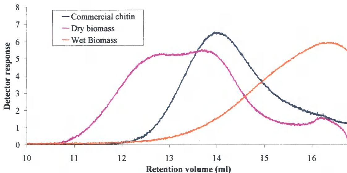
**Figure 4.51 - Refractive index trace produced by the GPC analysis of commercial chitin (Sigma), the purified solid A extracts from 'wet' and dry biomass using 5 % (w/v) LiCl:DMAc as the solvent and eluent.**
