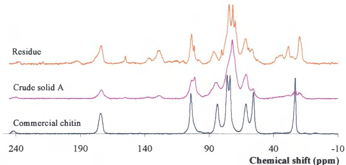
**Figure 4.41 -  $^{13}\text{C}$  CPMAS ssNMR spectra of commercial chitin (Sigma), the crude solid A from the chemical extraction procedure two and the acid insoluble residue remaining from the purification of the crude solid A.**
