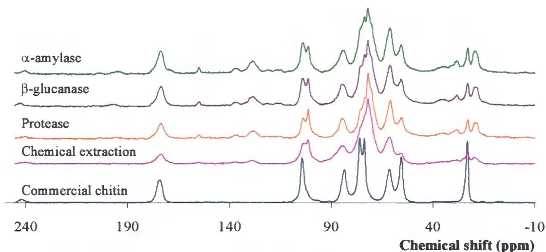
**Figure 4.44** -  $^{13}\text{C}$  CPMAS ssNMR spectra of solid A, chitin containing, samples extracted from the dry biomass by the chemical extraction procedure after incubation with a series of hydrolytic enzymes. The spectra of a commercial sample of chitin (Sigma) and a standard chemical extract are shown for comparison.
