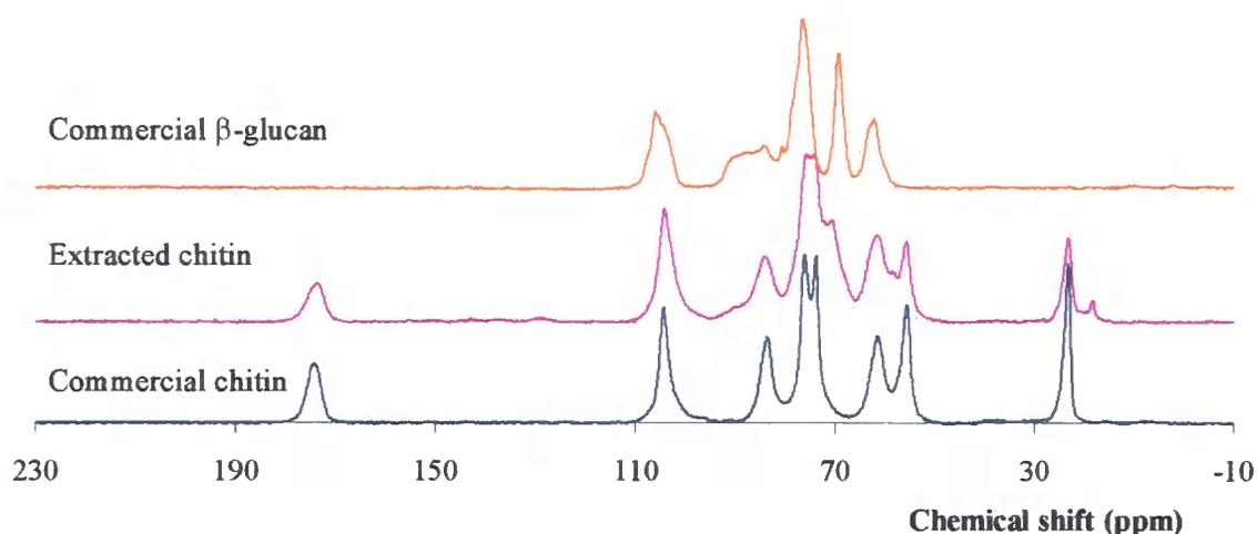
**Figure 3.14** -  $^{13}\text{C}$  CPMAS ssNMR spectra of chitinous material extracted from a fungal source, as described in sections 7.4.3 and 7.4.4, in comparison to commercial sources of chitin and  $\beta$ -glucan.
