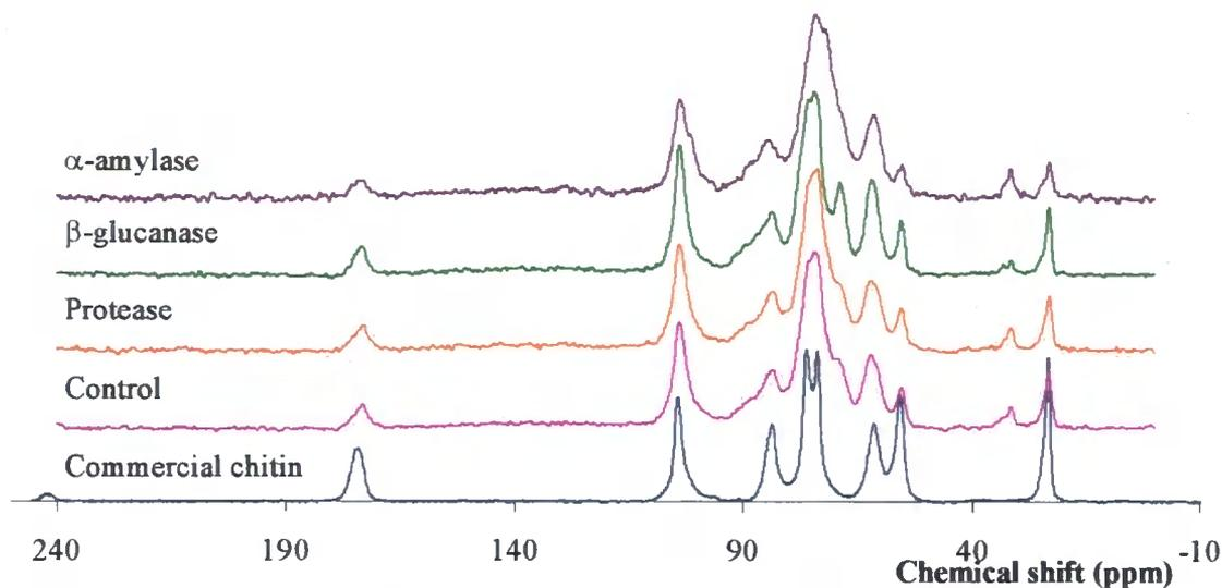
**Figure 4.55 -  $^{13}\text{C}$  CPMAS ssNMR spectra of crude chitin extracted by the standard chemical procedure from wet biomass which was cultured in the presence of the stated hydrolytic enzymes. The spectrum of a commercial sample of chitin (Sigma) is shown for comparison.**
