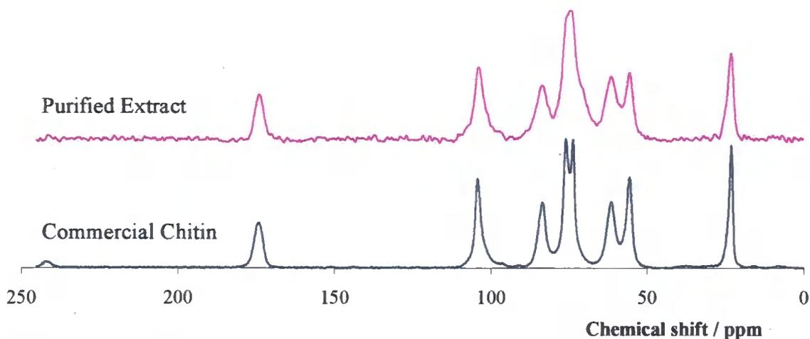
**Figure 5.65 -  $^{13}\text{C}$  CPMAS ssNMR spectra of purified chitinous material extracted from mycelia cultured in medium D ( $(^{15}\text{NH}_4)_2\text{SO}_4$ ) and a commercial chitin sample.**
