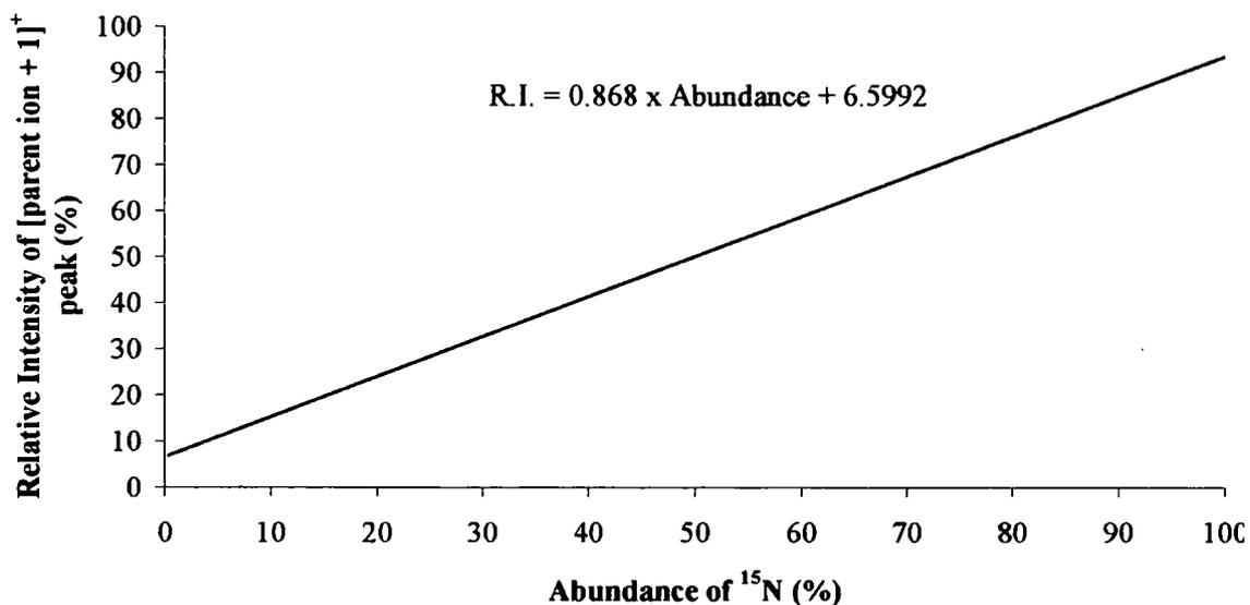
**Graph 5.9 - Standard curve of the theoretical relative intensity of  $[\text{M}+2]^+$  peak against abundance of  $^{15}\text{N}$ . Assuming natural abundances of 1.1 and 0.36 % for  $^{13}\text{C}$  and  $^{15}\text{N}$  respectively.**
