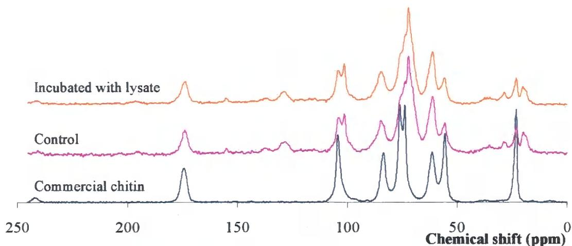
**Figure 6.81** -  $^{13}\text{C}$  CPMAS ssNMR of the crude solid A, chitin, extracted from dry biomass incubated in a buffered solution and in a buffered solution containing the lysate of *Mucor rouxii*. The spectrum of commercial chitin (Sigma) is shown for comparison.
