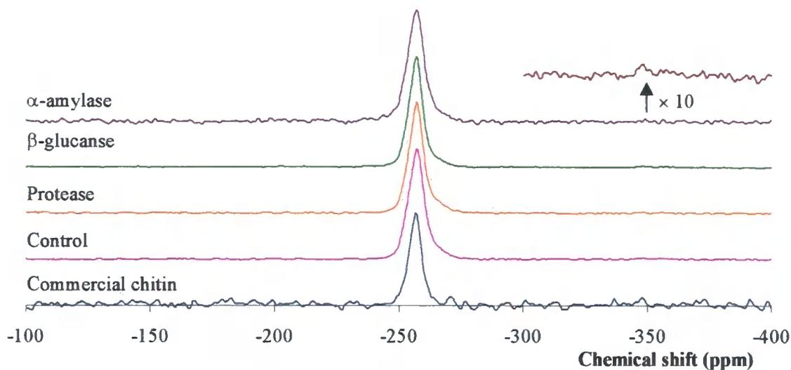
**Figure 4.54 -  $^{15}\text{N}$  CPMAS ssNMR spectra of whole 'wet' fungal biomass cultured in the presence of hydrolytic enzymes. The spectrum of commercial chitin (Sigma) is shown for comparison. The chemical shift range of  $-300$  to  $-400$  ppm of the  $\beta$ -glucanase spectrum is expanded by a factor of 10.**
