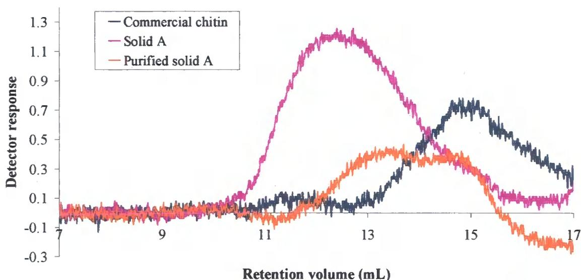
**Figure 4.42 - Refractive index trace produced by the GPC analysis of commercial chitin (Sigma), the crude solid A and the purified solid A using 5 % (w/v) LiCl:DMAc as the solvent and eluent.**
