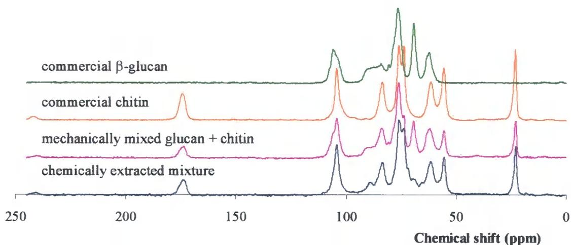
**Figure 3.13** -  $^{13}\text{C}$  CPMAS ssNMR spectra of a mechanical mixture of commercial chitin and  $\beta$ -glucan before and after chemical extraction. Spectra of the commercial chitin and  $\beta$ -glucan are shown for comparison.
