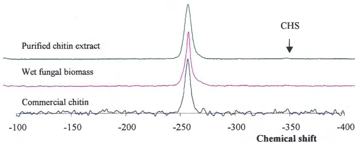
**Figure 5.76 -  $^{15}\text{N}$  CPMAS ssNMR spectra of the wet fungal biomass produced from the culture of the P2 strain of *P. chrysogenum* in  $^{15}\text{N}$  labelled conditions and the purified chitin extract. The spectrum of commercial chitin is shown for reference. CHS = the amino peak of deacetylated units.**
