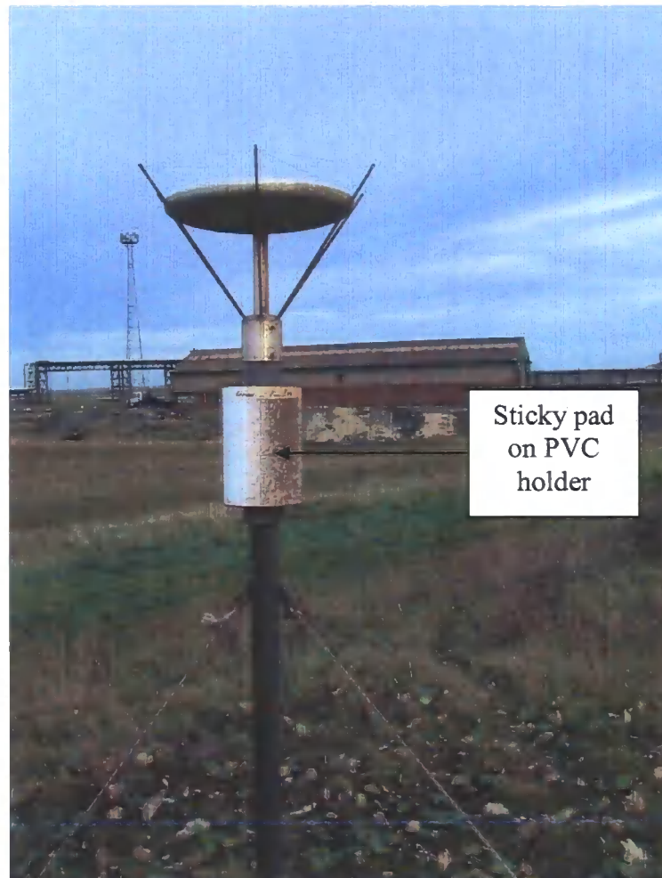
Figure 3.8 A cylindrical PVC sticky pad holder located on a tripod supporting the dry Frisbee deposition gauge.
