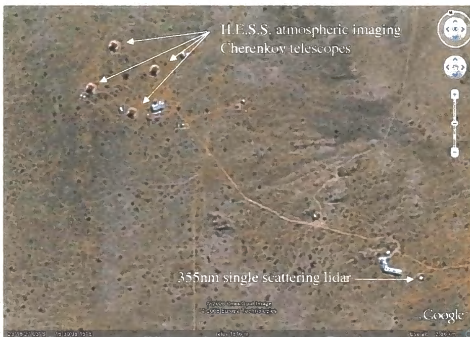
Figure 1.14: The H.E.S.S. site in the Gamsberg region of Namibia illustrating the square layout of the telescopes. The location of the lidar used for atmospheric monitoring is also highlighted on this map.
