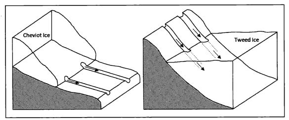
**Figure 49:** Model of Type B Channel formation. (a) Channels formed in a proglacial setting by runoff from the Cheviot Ice Cap, (b) Channels Formed as submarginal and subaerial water (and possibly Cheviot ice cap runoff) plunge directly beneath the TIS margin.
