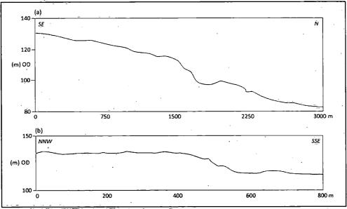
**Figure 52**: Channel long profiles. (a) Buxley Channel in the Lammermuir Hills (channel no. 2 in Fig.47, page 64); (b) Kings Chair Channel in the Cheviots (channel no.3 in Fig. 46, page 63). Note undulating sections.
