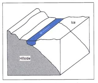
the position of the ice margin during *Figure 48:* Model of ice-marginal channel formation. Ice margin is retreating, cutting channels at retreat (Glasser and Bennett, 2004). The progressively lower altitudes.
