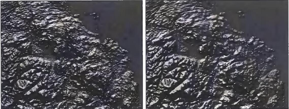
**Figure 13:** DEMs of field site **LEFT:** DSM of the area around Wooler **RIGHT:** DTM of the same area. Note the flat area in the centre of the image (The Milfield Plain) is 'smoother' in the DTM – artefacts such as trees and buildings have been removed (NEXTmap® Britain, Intermap Technologies, 2008)
