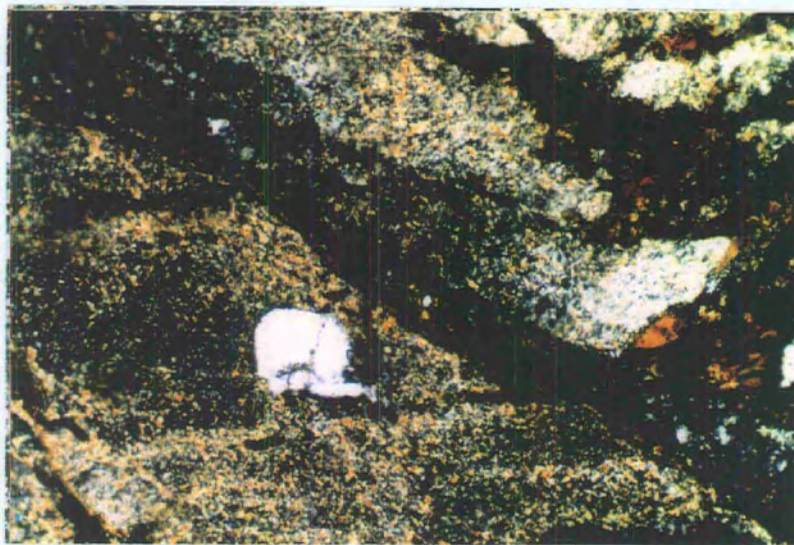
Plate 6.3 'Cataclasite' seam (dark band oriented at c.45^\circ to long axis of photomicrograph) cross-cuts banded gneiss host rocks. Dark brown matrix comprises aggregates of ultrafine-grained quartz, feldspar, hornblende and opaque minerals. Note that feldspar grains preserved in the host rock have suffered partial alteration to fine grained sericite needles. Field of view 1.3 \times 0.77\text{mm} , crossed polars.
