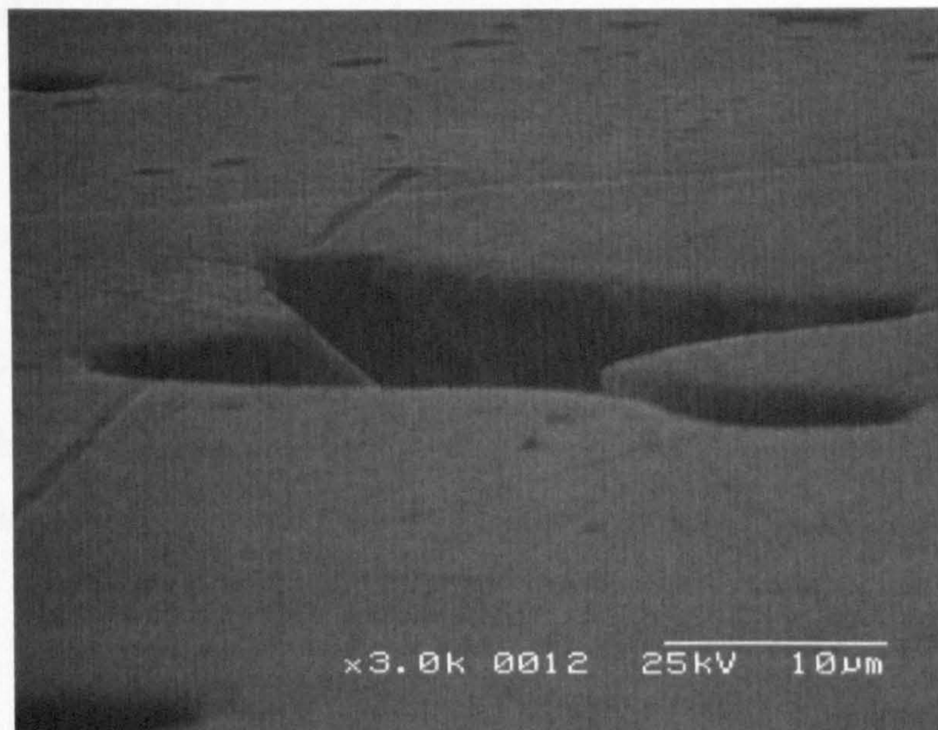
Figure 36 SEM image of a double heat treated specimen at 3 million cycles
