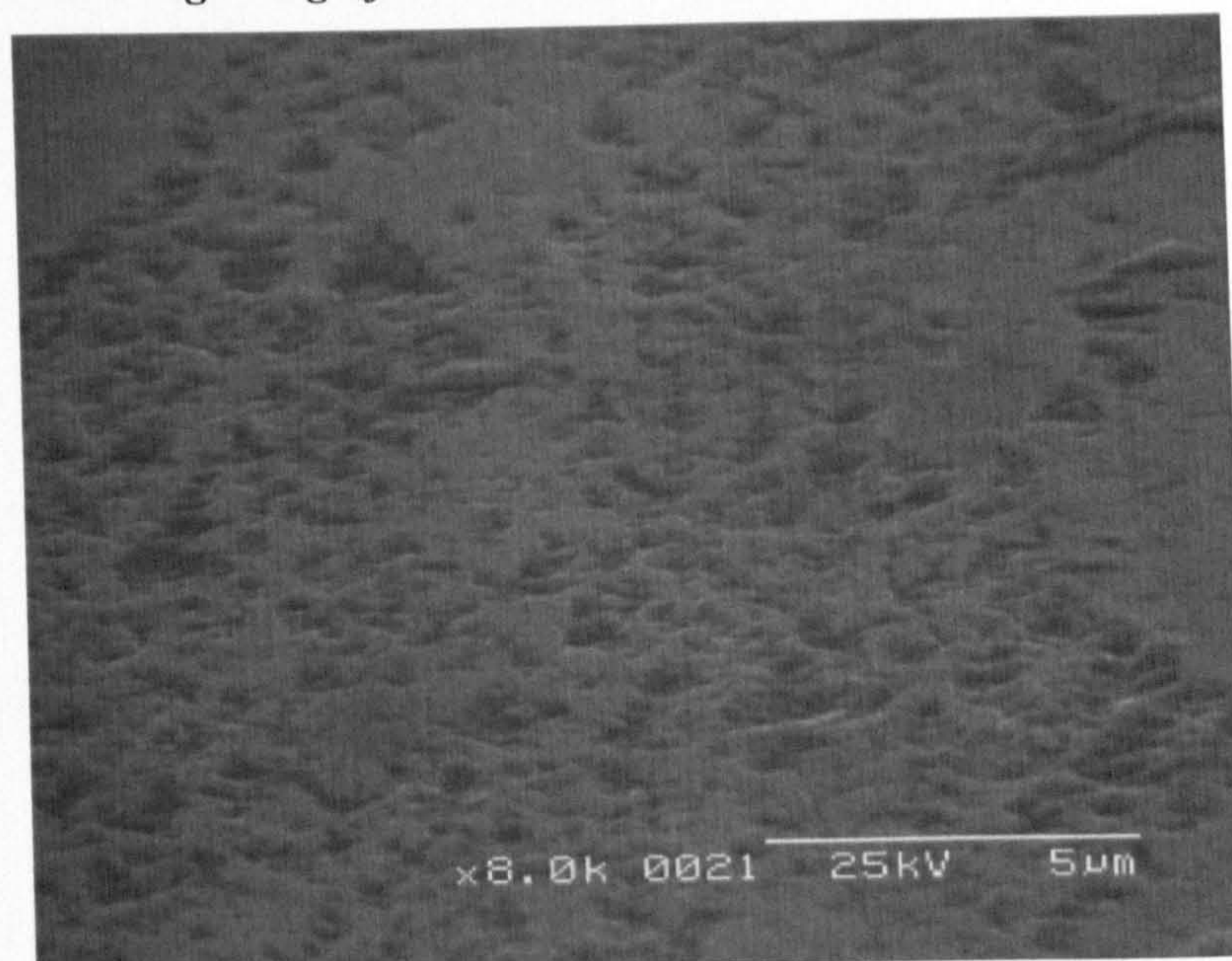
Figure 34 SEM high magnification image of as-cast specimen at 3 million cycles.
