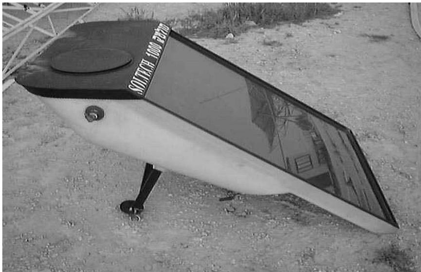
Figure 2.9f An Integrated collector–storage system [60].
