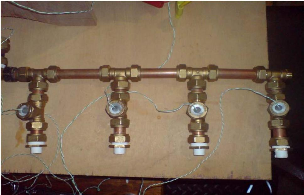
Figure 6.3a Manifold with thermocouples attached formed with compression fittings.
