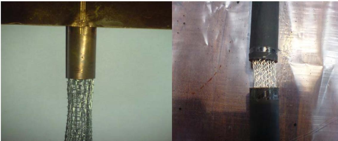
Figure 6.2e Porous medium inserted in a copper pipe.
