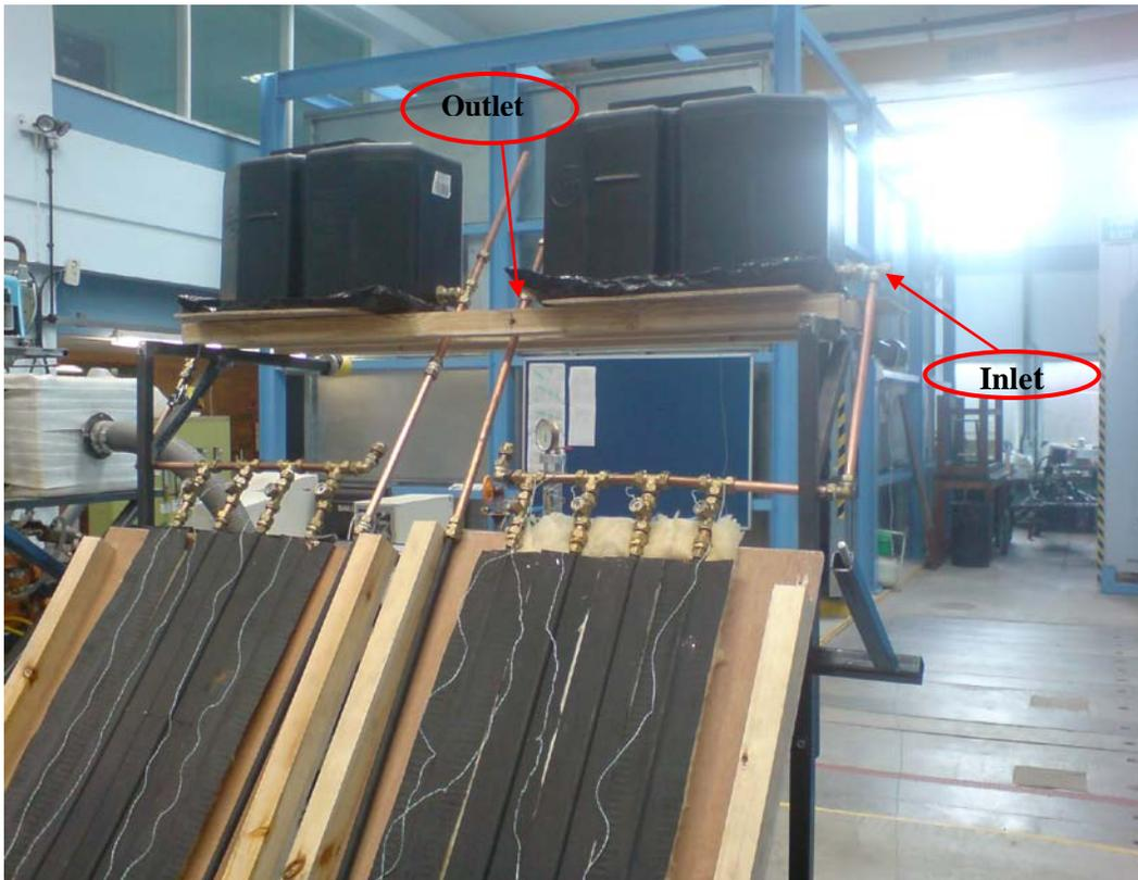
Figure 6.4b Water tanks connected to the collectors.
