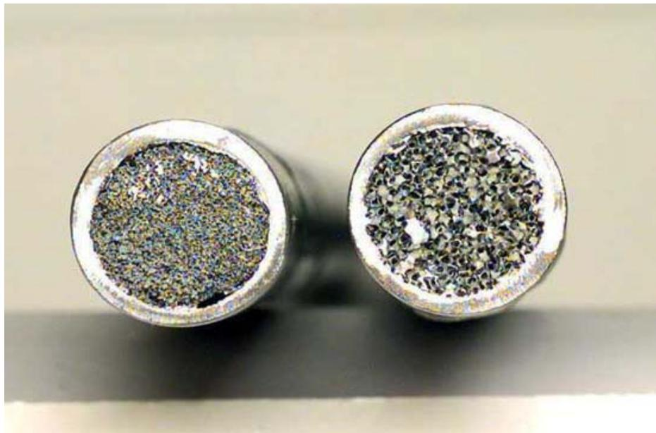
Figure 3.6e Metal-foam filled tubes [82].
