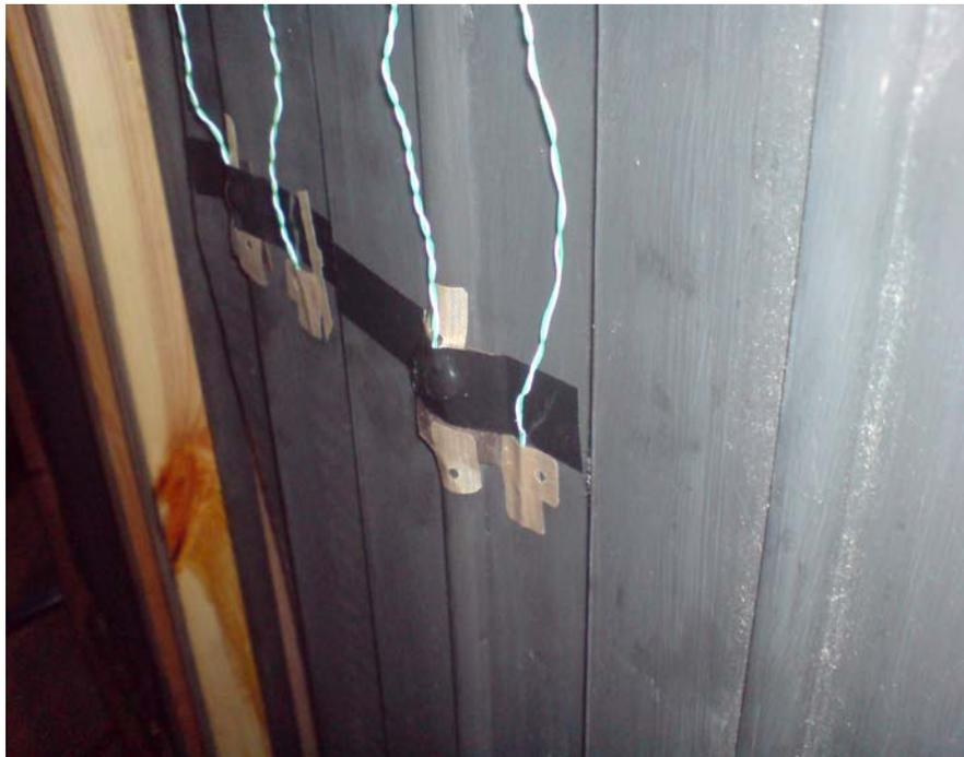
Figure 6.4j Surface temperature measurements setup.
