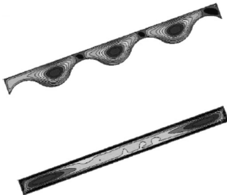
Figure 4.2c Temperature contours in the examined collectors.
