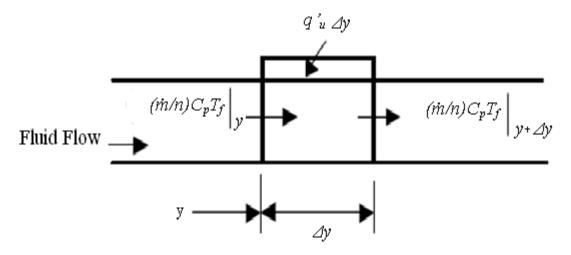
Figure 7.1a Energy balance on fluid element.
