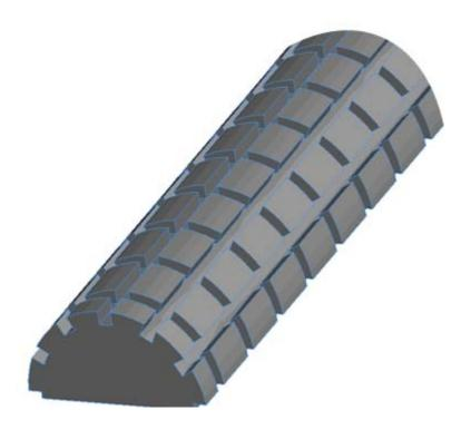
Figure 5.1i 3D geometry of the water domain in the heating pipe.
