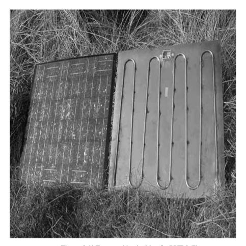
Figure 2.9j Front and back side of a PVT [67].
