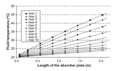
Figure 3.6c Fluid temperature in the tubes [74].
