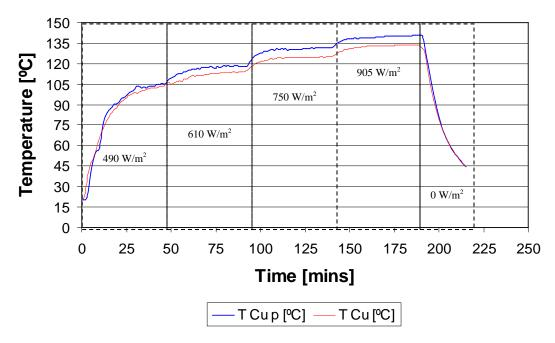
Graph 6.4.4c Temperature versus time at the exit of the copper finned pipes
