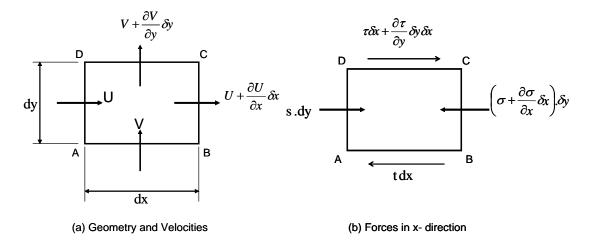
Figure 4.3a, b Flow in the control volume.
