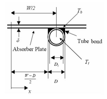
Figure 3.13a Fin and Tube dimensions.
