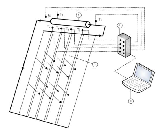
Figure 6.3d Schematic of the experimental Setup.
