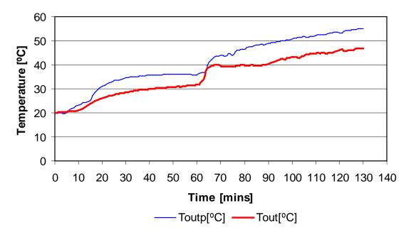
Graph 6.2.1a Temperature of the water in the outlet of solar panels as a function of time.
