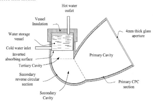
Figure 2.9h An inverted absorber ICSSWH [62].
