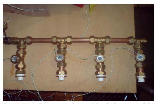
Figure 6.3a Manifold with thermocouples attached formed with compression fittings.
