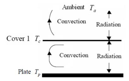
Figure 3.11a Heat transfer mechanisms through a collector with a single cover.
