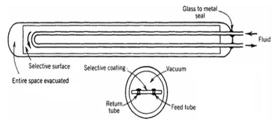
Figure 2.4b Direct evacuated tube Flow collector.
