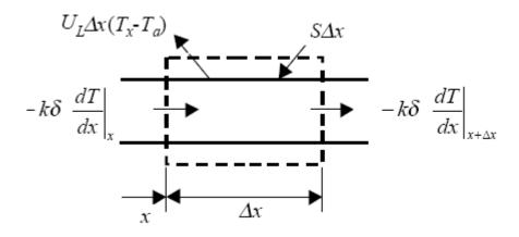
Figure 3.13c Energy balance on fin element.
