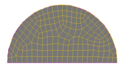
Figure 5.2b Quad-Pave meshing scheme for the cross-sectional area in the tubes.
