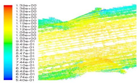
Figure 5.5d Velocity vectors in the profiled pipe design.
