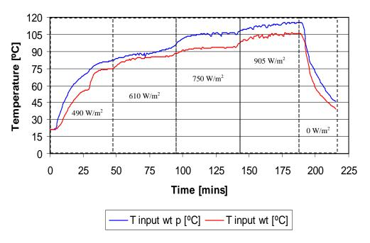
Graph 6.4.4e Temperature versus time at the inlet of the water tanks.
