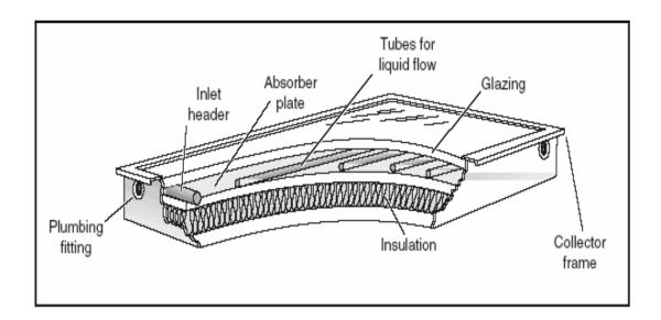
Figure 2.2a Flat plate solar water collector [9].
