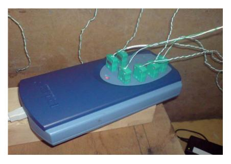
Figure 6.2h Data logger with thermocouples attached.
