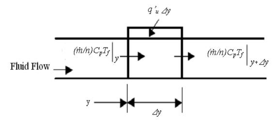
Figure 3.13d Energy balance on fluid element.
