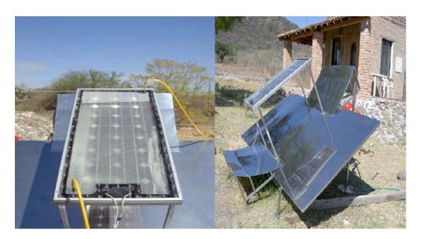
Figure 2.9k A bifacial PV module [69].
