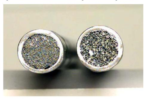
Figure 3.6e Metal-foam filled tubes [82].
