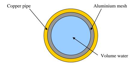
Figure 5.5a Cross-section of a pipe with aluminium mesh.
