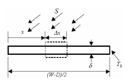
Figure 3.13b Energy balance on fin element.
