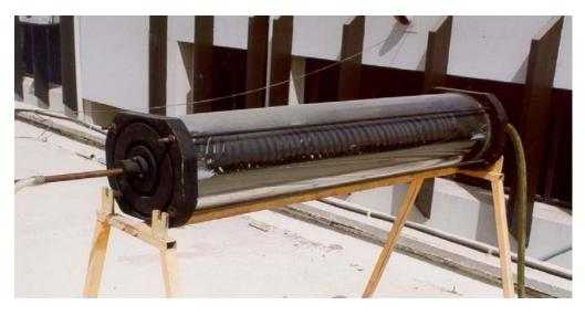
Figure 2.9i A cylindrical solar water heater [63].
