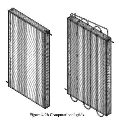
All turbulence models (solution options depending on the type of flow laminar or turbulent) available in FLUENT were tested (variations of  $k-\epsilon$  and  $k-\omega$ , Reynolds stress model and Spallart–Almaras model), for steady state conditions, and the standard  $k-\omega$  was proven as the most appropriate.
