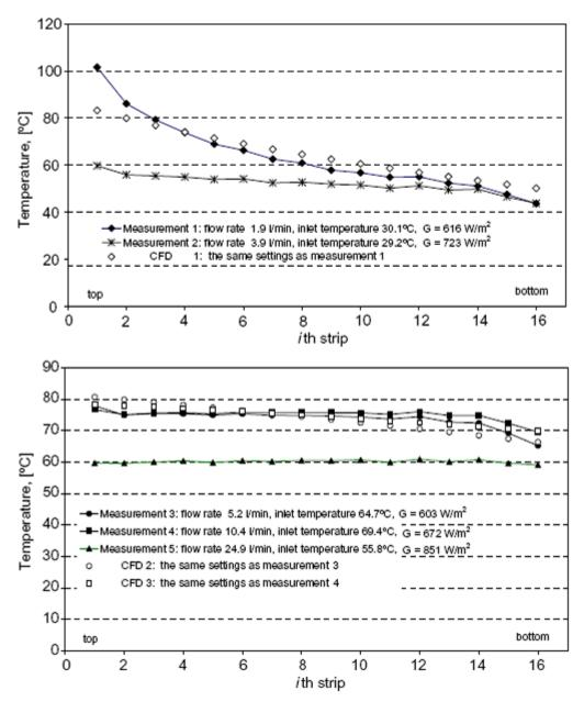
Figure 3.6a Fluid temperature at different flow rates [73].
