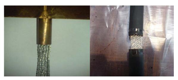
Figure 6.2e Porous medium inserted in a copper pipe.
