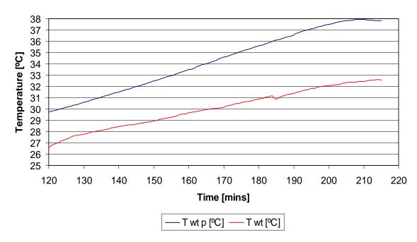
Graph 6.4.4f Temperature versus time inside the water tanks.
