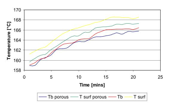
Graph 6.4.4a Temperature versus time at the surface of the collectors.
