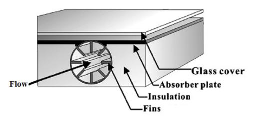
Figure 2.91 Solar water heater with internal fins [117].
