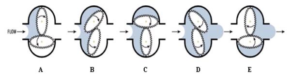
Figure 6.4h Mass Flow meter operating steps.
