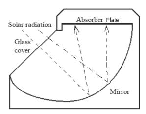
Figure 2.9c Inverted Absorber Plate [56].
