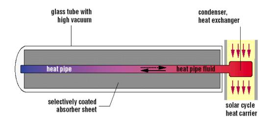
Figure 2.4c An evacuated tube collector with heat pipe.
