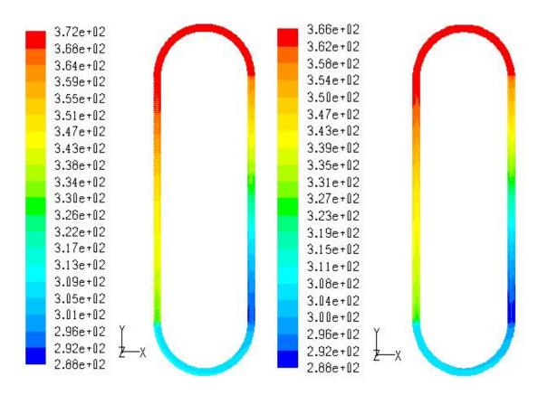
Figure 5.4a Temperature contours of both geometries (K).
