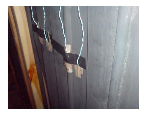
Figure 6.4j Surface temperature measurements setup.
