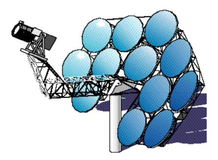
Figure 2.6b Two-axis tracking parabolic dish collector [14].
