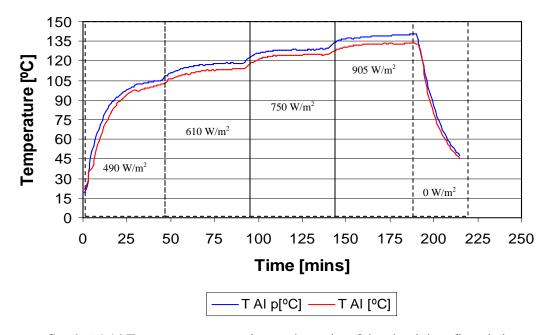
Graph 6.4.4d Temperature versus time at the outlet of the aluminium finned pipes.
