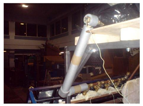
Figure 6.4c Insulated water tanks and copper pipes.
