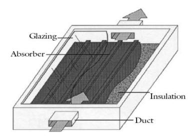
Figure 2.3a Flat Plate Air Collector [9].
