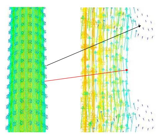
Figure 5.4f Velocity vectors inside the pipe with metallic mesh insertion.
