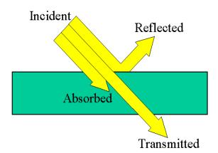
Figure 3.2d Radiation process.
