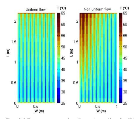
Figure 3.6b Temperature contours for uniform and non-uniform flow [74].
