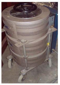
Figure 6.2d A three phase electrical transformer.
