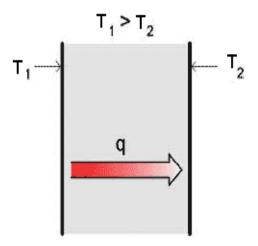
Figure 3.2a Conduction process.
