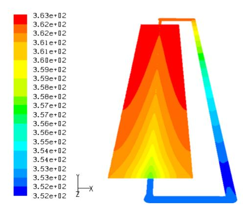
Figure 5.5b Simulated collector section.
