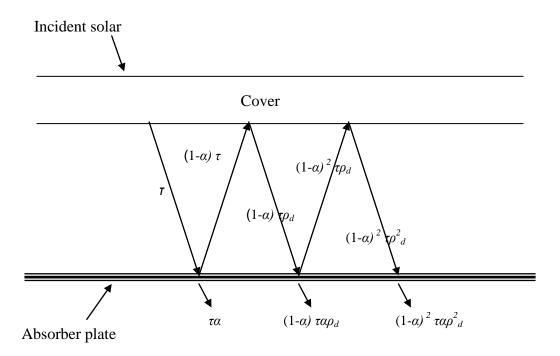
Figure 3.7a Absorbed solar radiation under a cover system.
