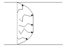
Figure 3.3b Turbulent flow.
