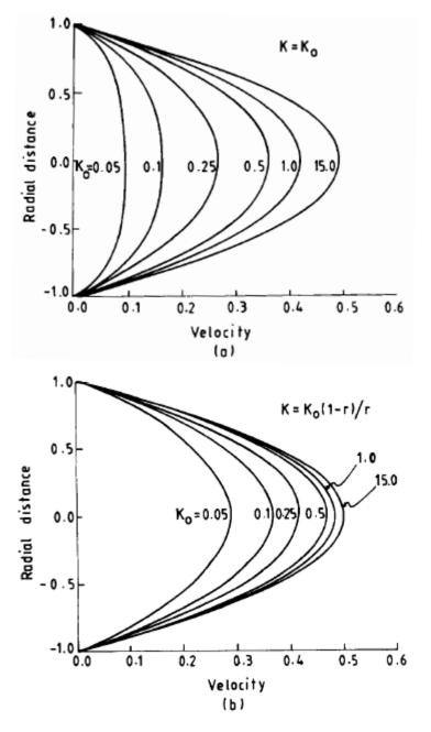
Figure 3.6d Velocity distribution for different values of K<sub>o</sub> [79].
