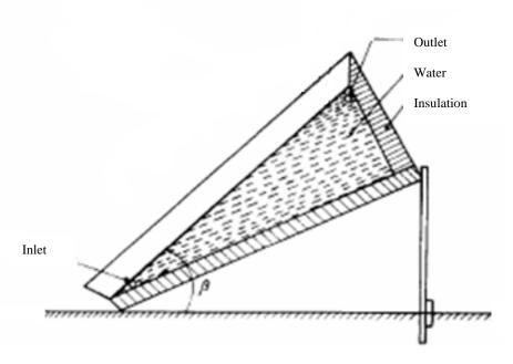
Figure 2.9d A triangular built-in-storage solar water heater [58].
