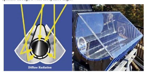
Figure 2.5a Stationary concentrating collectors.
