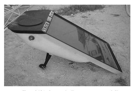
Figure 2.9f An Integrated collector-storage system [60].
