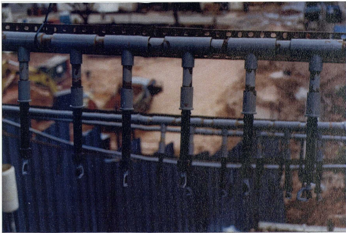
Figure 3.24 Microsprays manufactured by Netafim that were used in the rainfall simulator.
