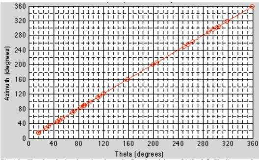
Fig. 4.9 The plot of azimuth against the angle  $\theta$  at the minimum RMS of  $\theta$ . The line was found to have the gradient value 1 and the y-intercept -0.006. The pixel position of the zero-azimuth used for the plot was (254, 196).
