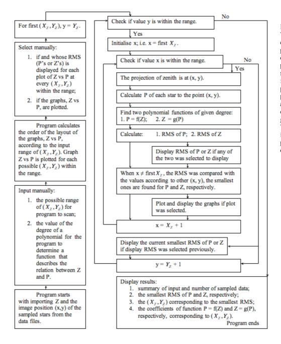
Fig. 4.6 The flow chart of the process of the computer programme. It shows what functions the programme performed and what output it generated. The arrows indicate the process direction.
