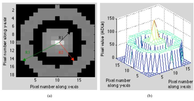
Fig. 5.3 The image of star Alioth in (a) and the corresponding 3-D plot in (b). In (a), the star's image is presented in the centre aperture and the grey annulus shows the brightness of sampled sky. The dark area, showing zero counts, is the part of the image being taken away when sampling. R1, R2 and R3 indicate the radii of the aperture, inner and outer annulus, respectively. In (b) shows the flux strength on each part of the sample.
