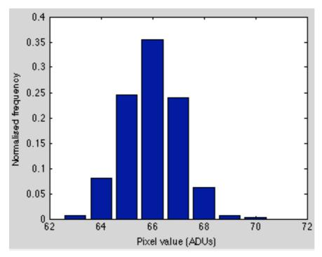
Fig. 5.6 Histogram of the normalised frequency of the pixel values within the sampled sky patch. The graph shows a mode at 66 ADUs and the FWHM of the distribution is 2.591.
