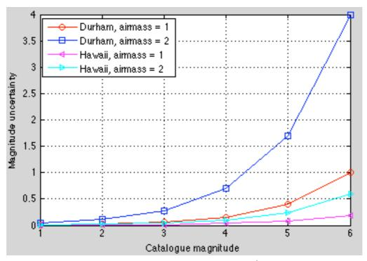
Fig. 5.15 The plot of magnitude accuracy of the stars of 1<sup>st</sup> to 6<sup>th</sup> magnitude determined in Hawaii in contrast to in Durham.
