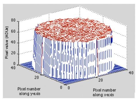
Fig. 5.5 The 3-D plot of the flux of a patch of the sky. It centred at the pixel position (241, 269) on the frame captured at 22:00 on 4 April 2008, and had a radius of 20 pixels, so around 1200 pixels were sampled.
