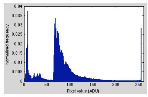
Fig. 5.2 The histogram of the flux of the all sky image taken at 22:00 on 4 April 2008. The dark counts were subtracted from the total counts before plotting.
