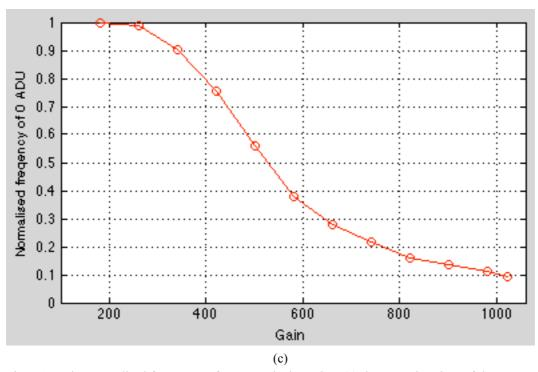
Fig. 2.3 The normalised frequency of 0 ADU pixels against (a) the operating time of the camera, (b) the exposure time and (c) the gain parameter, respectively. These graphs show how the number of the unaffected pixels by the dark currents changed with each setting parameter.
