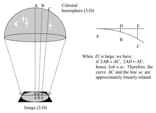
Fig. 4.2 The schematic representation of mapping from 3-D celestial hemisphere onto the 2-D image plane. The dash lines represent the light rays and the arrows indicate their travelling directions. The points A and a represent the sky position and image position of zenith, respectively. The points A, B and C locate on the same great circle of the celestial sphere. The points b and c are the image positions of B and C, respectively.
