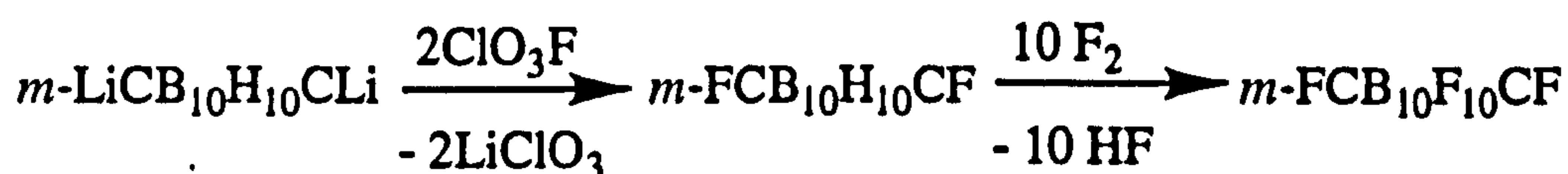
scheme 2.17: fluorination reactions of ortho, meta and para-carboranes
