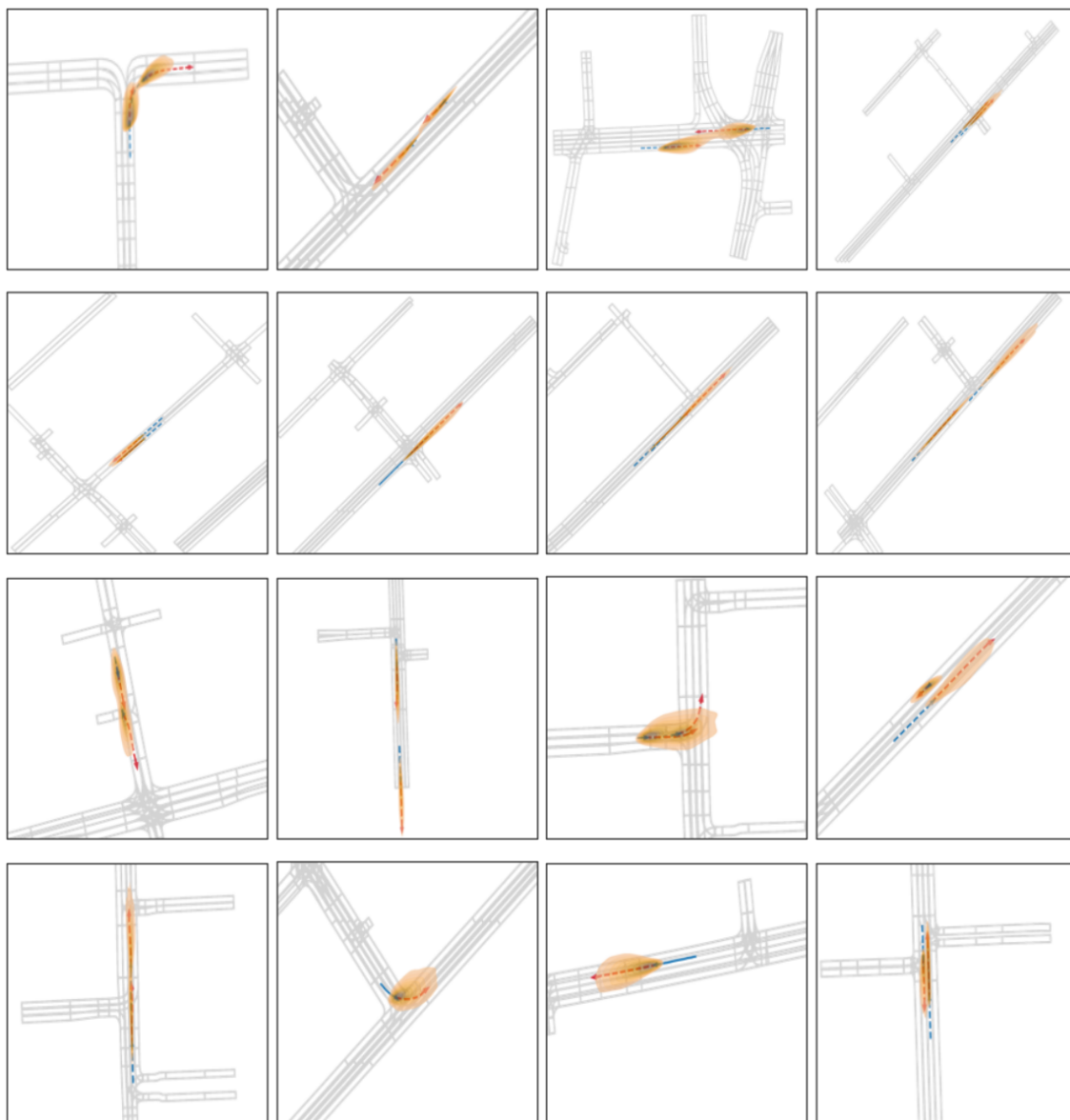
Figure 5.10: Predicted trajectory distributions using the proposed BP-SGCN on the Argoverse 1 dataset. Past trajectories are shown in blue, ground-truth trajectories in red, and predicted trajectory distributions in orange.
