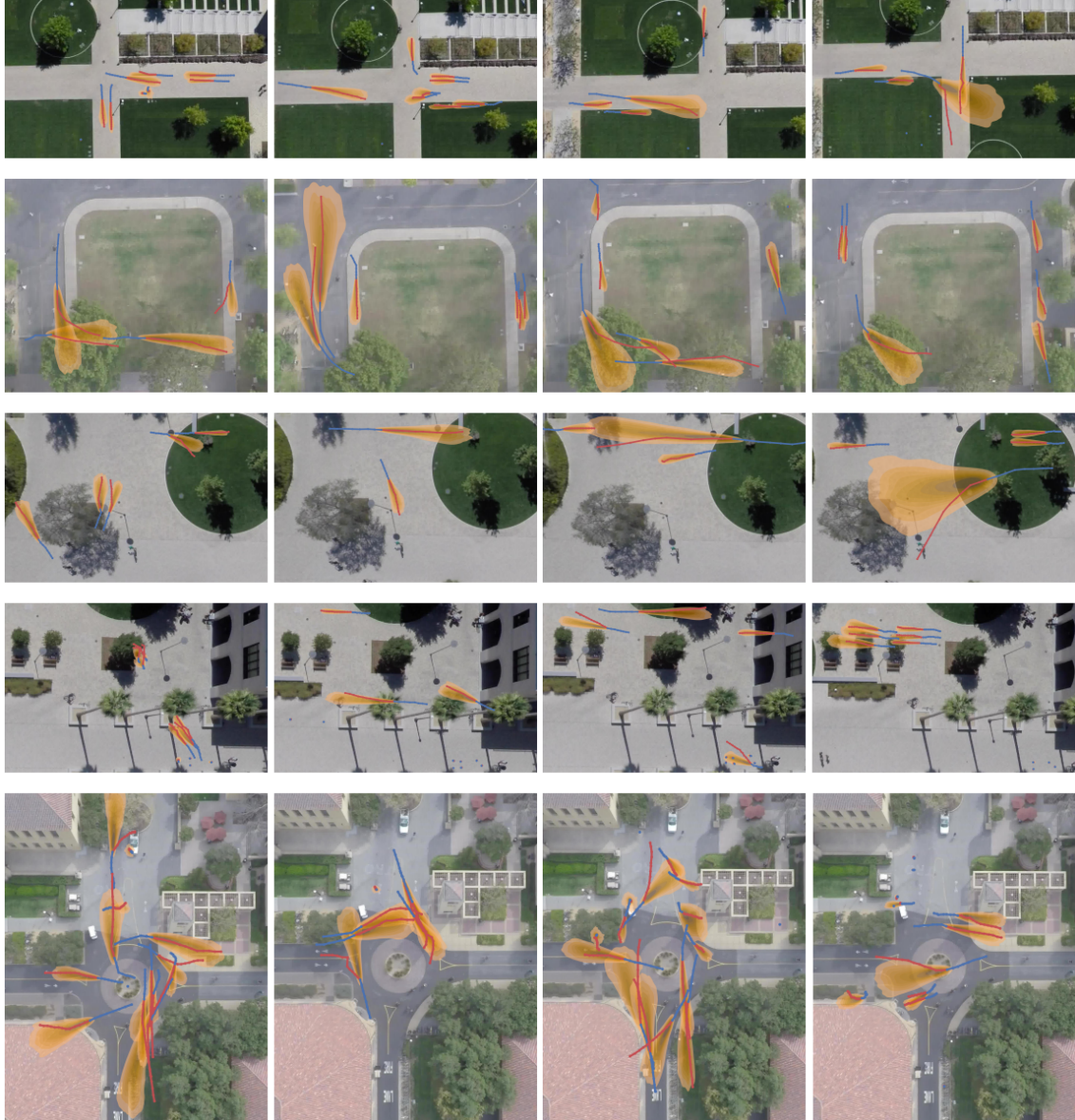
Figure 5.9: Predicted trajectory distributions using the proposed BP-SGCN on the SDD dataset. Past trajectories are shown in blue, ground-truth trajectories in red, and predicted trajectory distributions in orange.
