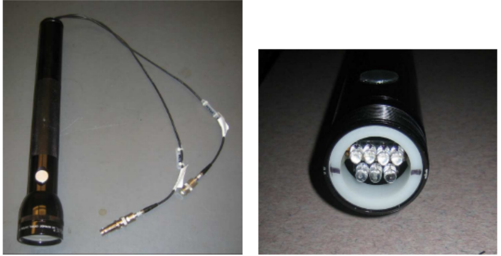
Figure 2.9: VERITAS LED based calibration system housed in a modified Maglite with diffuser and trigger input ( left ). Arrangement of the seven LEDs inside the housing ( right ) [77].
