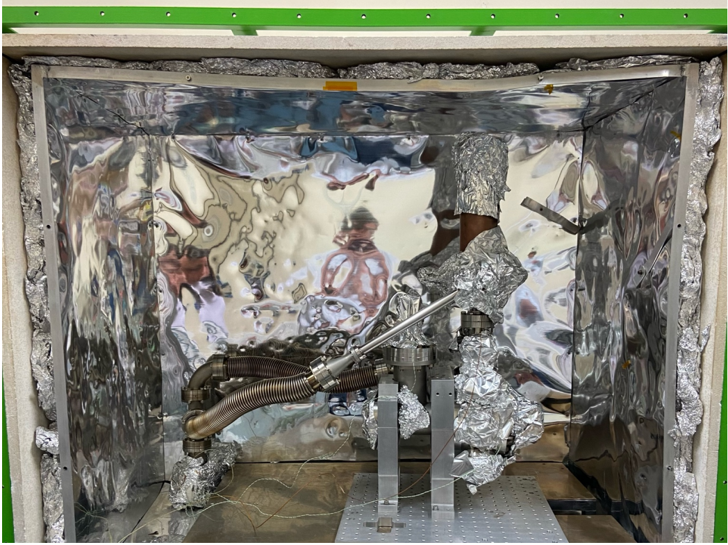
Figure 5.1: Experimental vacuum system during pump down and bake-out. The system is shown inside a bakeout oven with external heater tapes and thermocouples attached. The vacuum chamber is connected to the external pumping rig via flexible bellows and DN40CF flanges. Tin foil is used to minimise temperature gradients across the chamber, especially at glass and glass-metal interfaces, to prevent stress induced cracking. The pumping rig (not pictured) sits beneath the oven.
