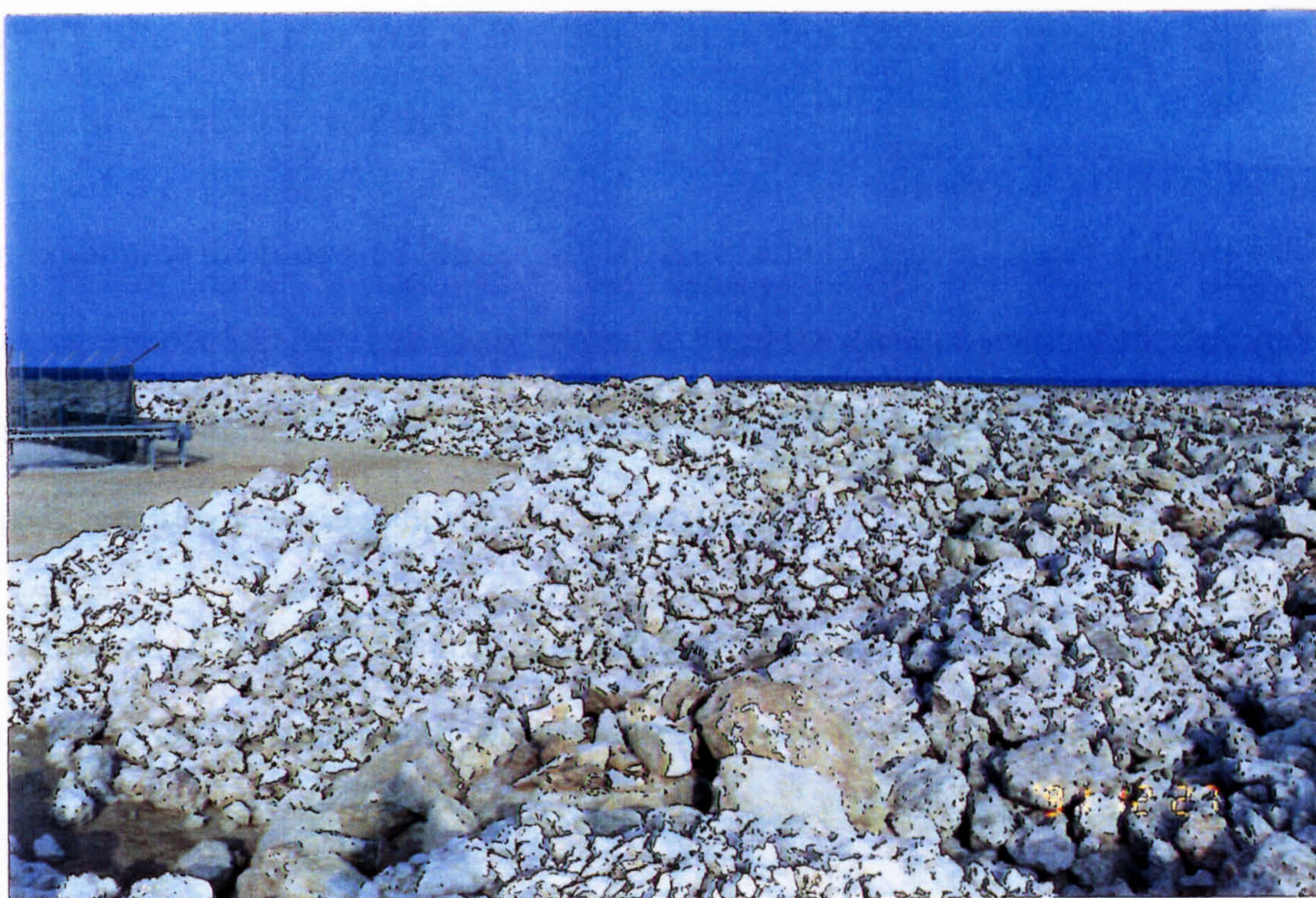
Plate 5.10: Stones collected at Ras Laffan during pipelaying for the gas lines between Ras Laffan and Umm Said. The stones will be used for land reclamation.
