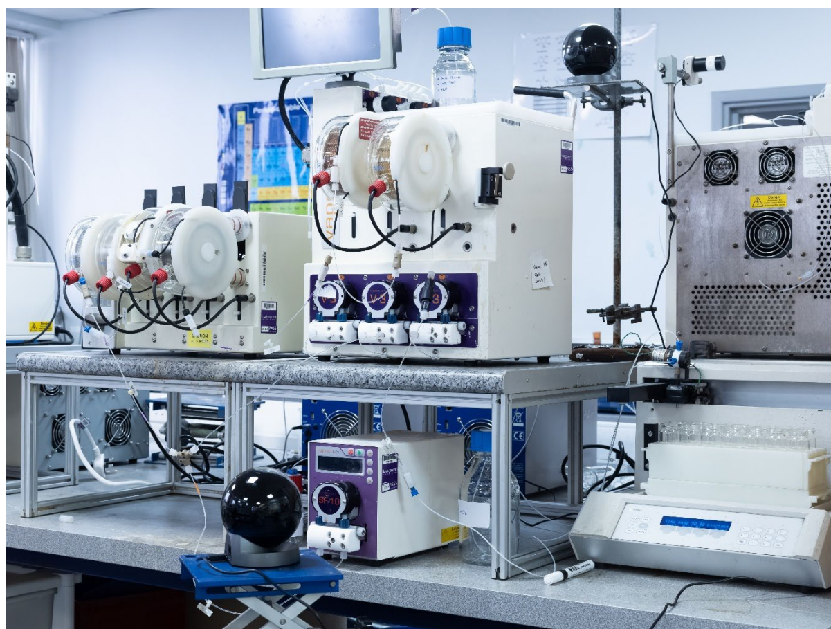
Figure 36. The flow set up with web cam monitoring and wifi smart plug to monitor overnight reaction.
