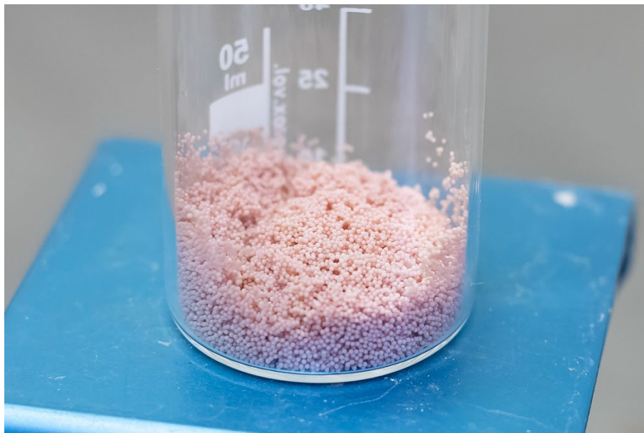
Figure 94. The heterogeneous base of Ambersep® 900 hydroxide form.
