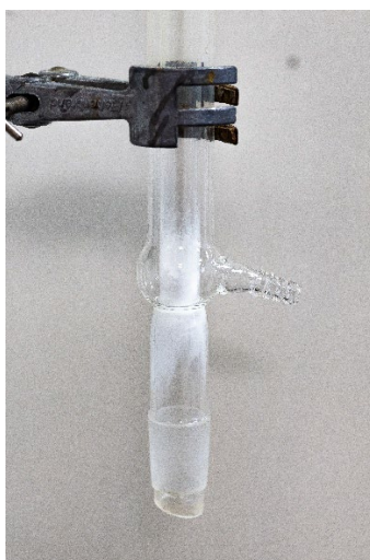
Figure 62. Paraformaldehyde subliming in the reflux condenser.
