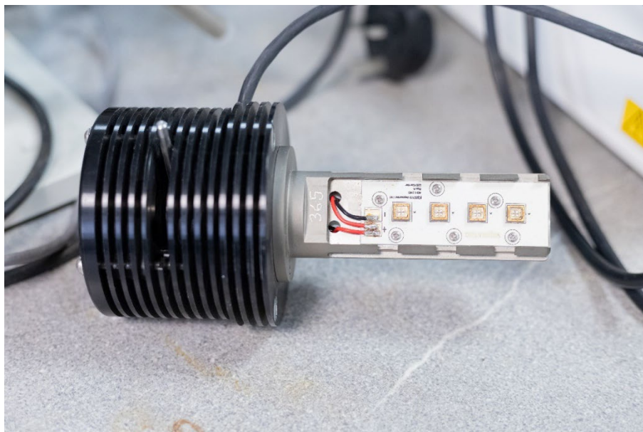
Figure 79. High power LED at 365 nm.
