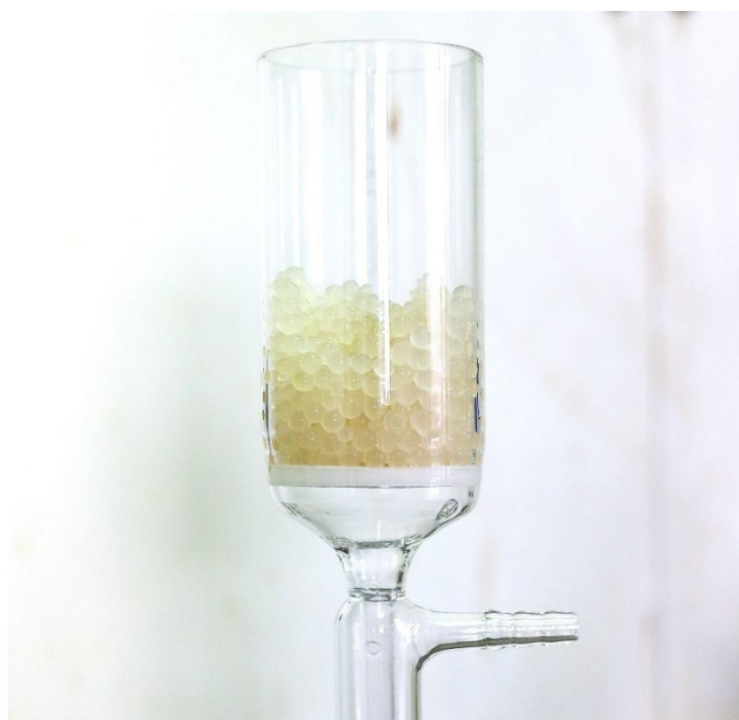
Figure 24. Filtered sodium alginate beads in Buchner funnel.
