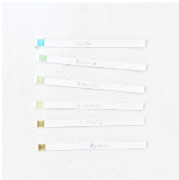
Figure 25. Glucose test strips at various times. Top to bottom: a to f, A. Lactose; B. just dissolved, C. >10 min D. >20 min, E. > 50 min, F. >90 min.
