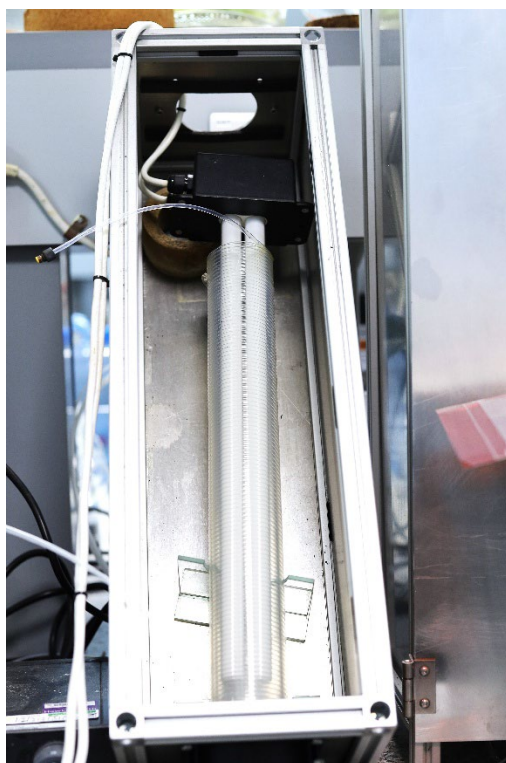
Figure 72. Interior look of the customised design of the photoreactor.
