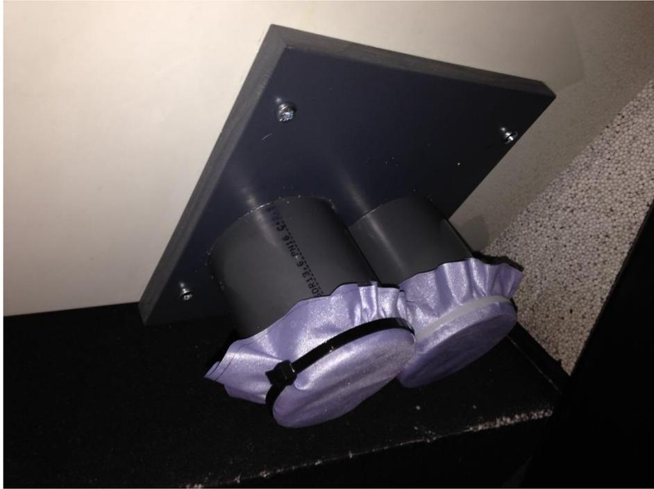
**Figure 3.12** Weather-proofed fabrics with super hydrophobic coating
