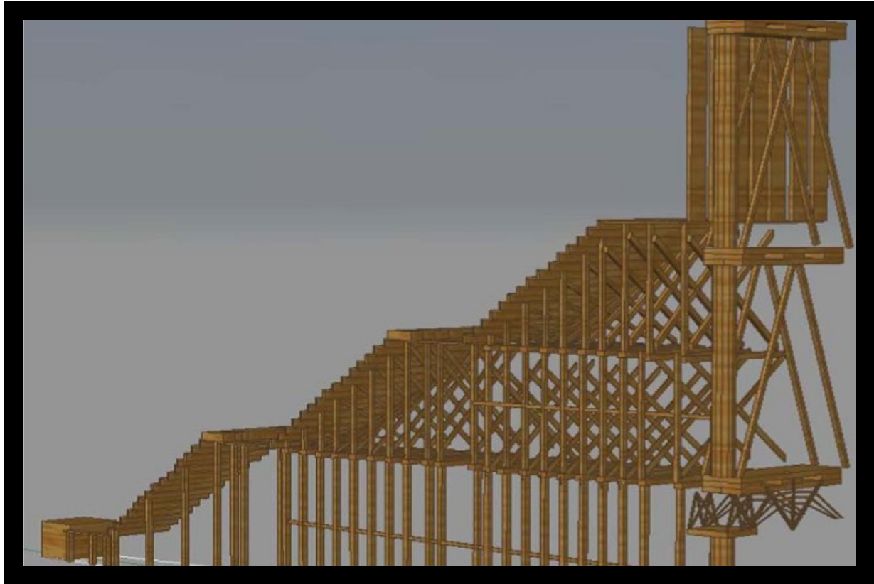
Figure 10 Cross-sectional view of a segment of the amphitheatre at Fidenae
