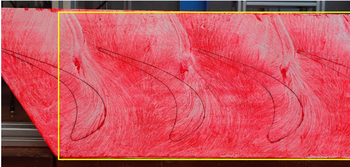
Figure 6.19 Surface flow visualization image of the test case
