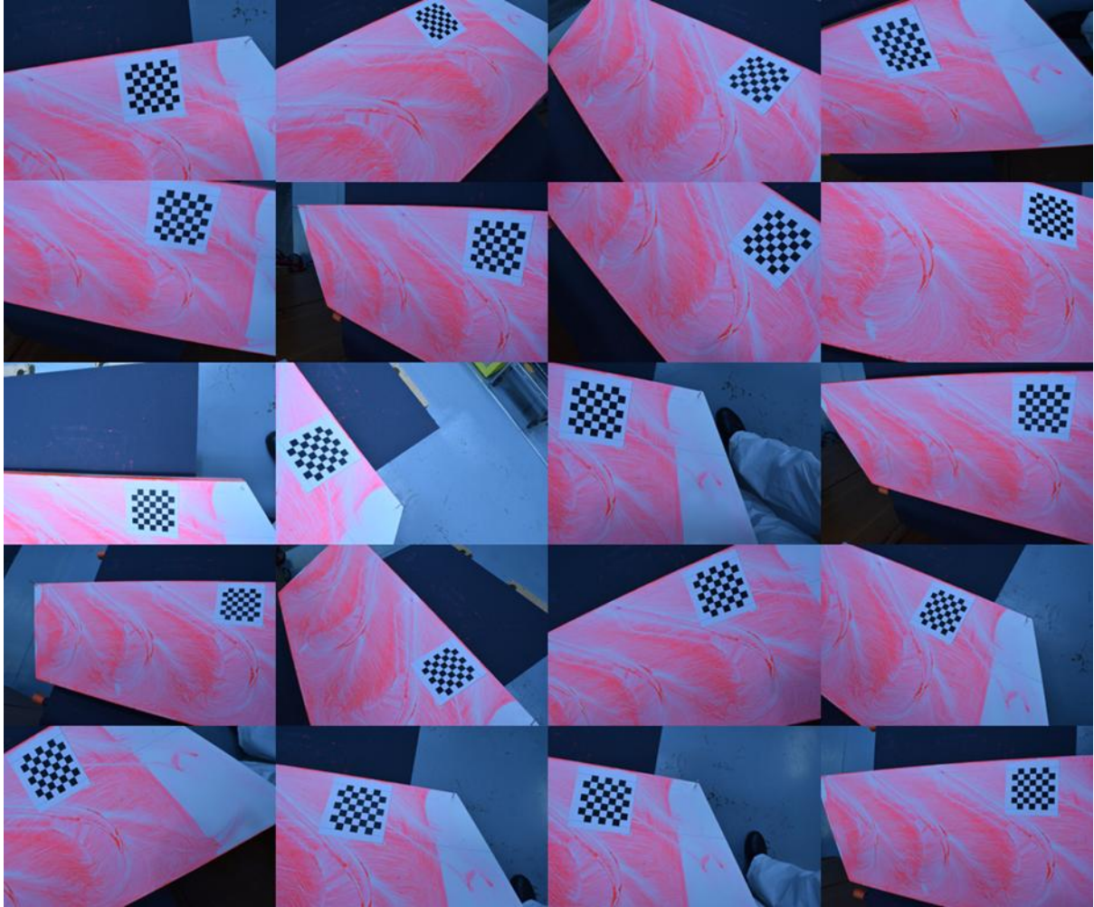
Figure 4.2 Images used for chessboard calibration
