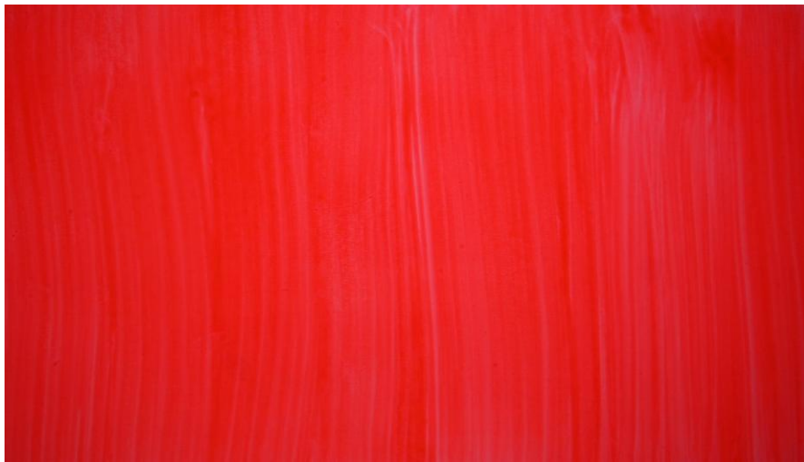
Figure 5.1 In the unobstructed test article area, evenly apply the oil/dye mixture using a brush
