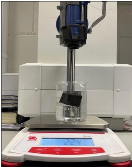
Figure 2.12. Density measurement setup. The picture shows a test sample suspended in distilled water and placed on a digital scale. This setup allows for the measurement of the sample's mass in the fluid to determine its density.
