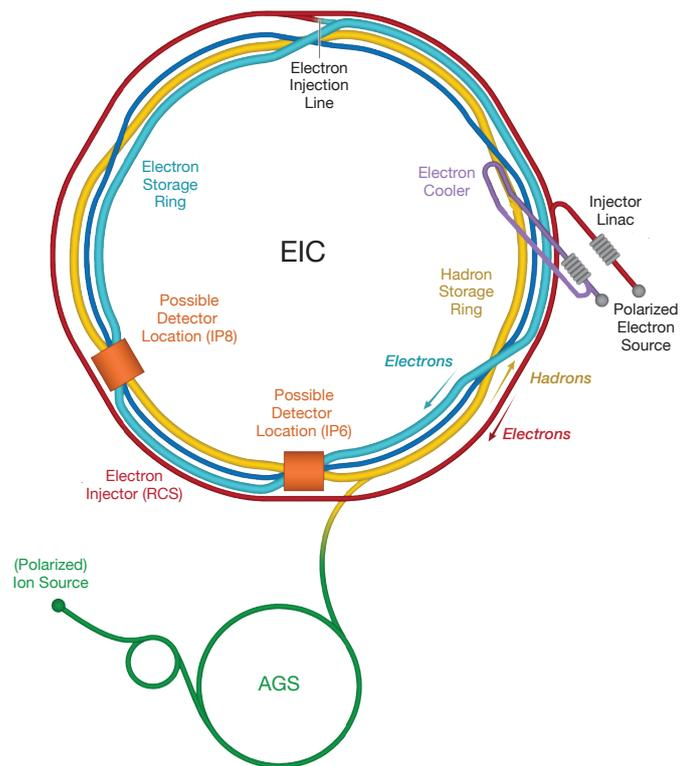
Figure 2.1: Sketch of the layout of the planned EIC, based upon the existing RHIC at BNL. Taken from [8].
