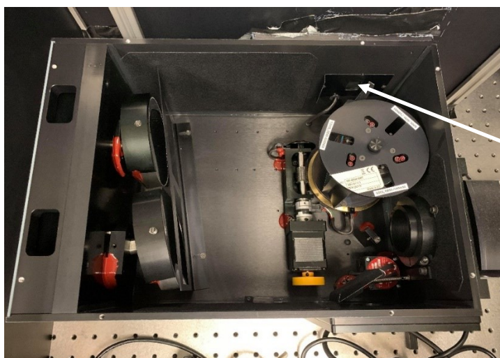
Figure A1.17: The inside of the spectrograph with any arrow where the torch was placed.
