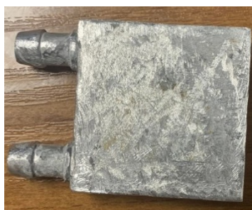
Figure 3.13: The water bath used for the cooling of the DRIFTS system.
