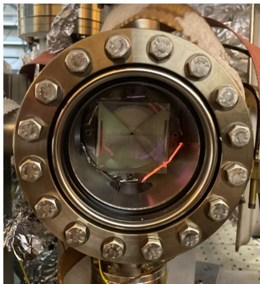
**Figure 3.7:** Incandescence of a set of Rb dispensers during activation. Pyramid MOT mirrors visible as the square object in the centre of the viewport. Other atom dispensers are arranged around the pyramid mirrors in a hexagonal formation.
