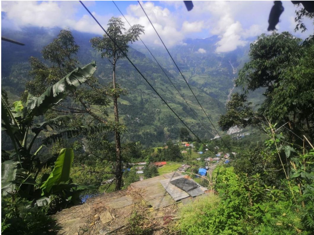
Figure 2: Drinking waterpipes elevated to prevent damage from slumps and landslides
