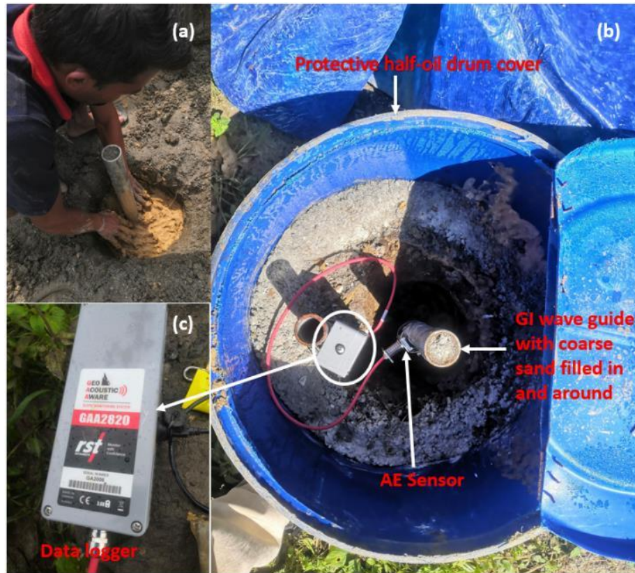
Figure 6.12: (a) Sealing the surface with bentonite, (b) AE sensor and its different parts, and (c) data logger
