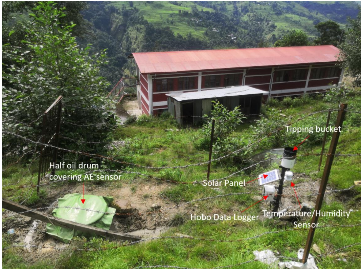
Figure 6.6: Landslide monitoring instruments installed at Tallo Sigarche (local primary school seen in front of the instruments)
