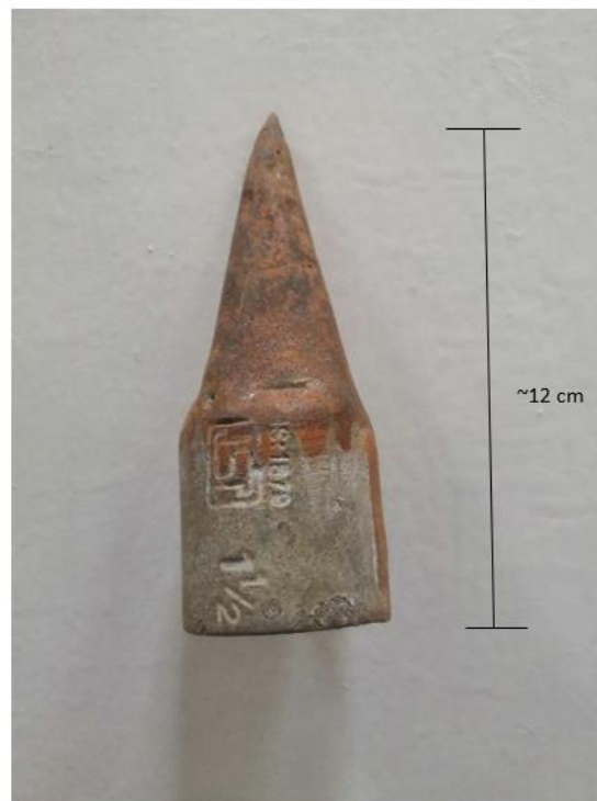
Figure 6.11: Conical end designed to seal the lower end of GI pipe/wave guide
