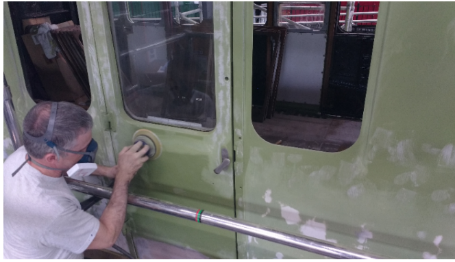
Figure 20. An expert painter/decorator is hired out to come paint the trains. He patches the holes, then comes back to sand them, then comes back to prime, then paint, then paint many more layers. After each time he comes to Locomotion, the work must stop until he is able to free up his schedule to come back for the next step. A reliance on his expertise is fundamental to the upkeep of the museum collection (Fieldwork photograph, Suarez Ferreira 2016).
