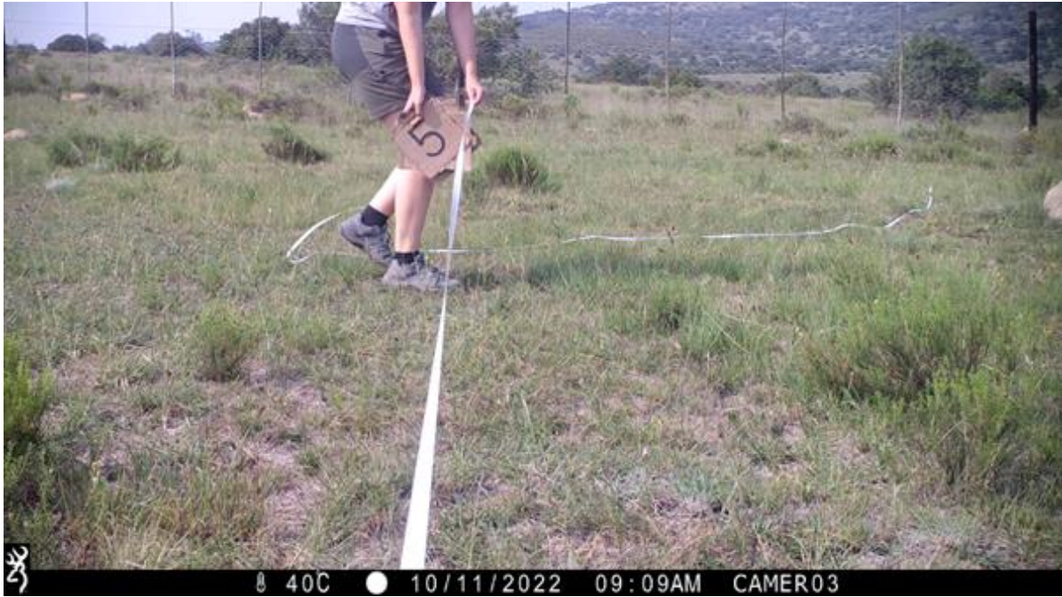
Figure 3. Screenshot from reference videos taken on collect of each camera trap, used to estimate radial distances from the camera to the midpoint of the detected animal. Image shows researcher walking across the camera field of view with a tape measure indicating 5m distance.
