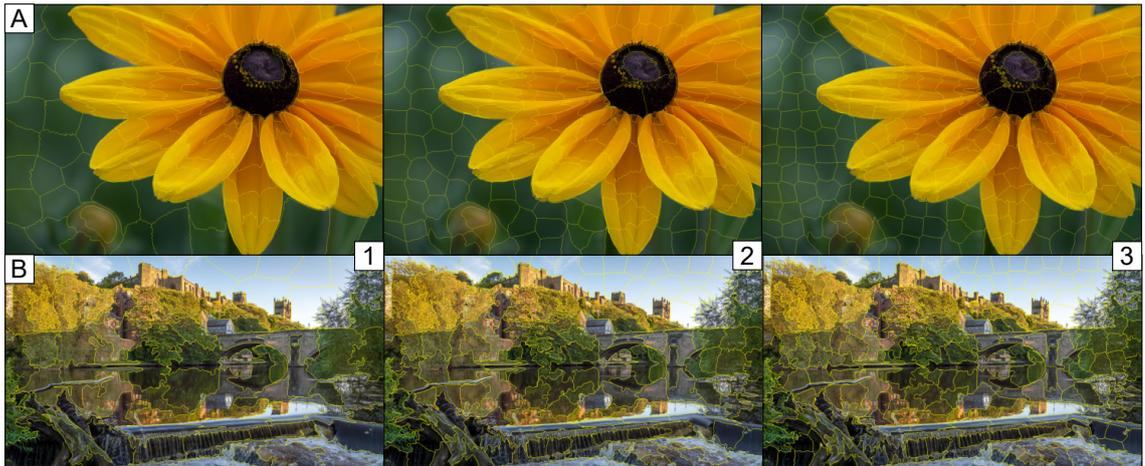
Figure 5.6: Example of Simple Linear Iterative Clustering (SLIC) [16] Superpixel Segmentation across flower (**A**) and Durham (**B**) using  $\sigma=5$  with number of segments as 100, 200, and 300 (**1**, **2**, **3**)
