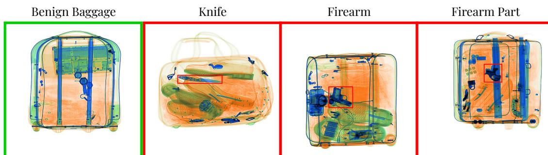
Figure 2.8: Examples from the University Baggage Anomaly (UBA) Dataset [2] outlining one normal sample (left) followed by three samples from anomalous classes: Knife, Firearm, Firearm Part.
