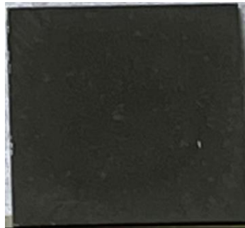
Figure 4.2 CZTS ink deposited on SLG substrate, 2.5 x 2.5 cm, via spin coating technique.
