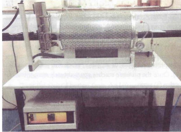
Figure 4.3 The furnace used for sulphurisation (annealing system) showing the arrangement of the horizontal tube furnace and the gas flow control system.
