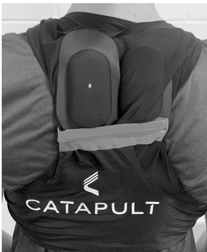
Figure 6.2: Placement of GNSS Devices
